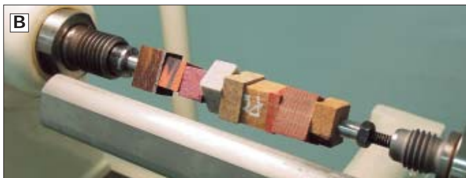
B You'll save time by rough-turning an assortment of centerbands at once.
