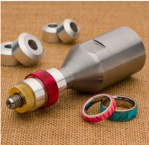
Mandrel for holding ring blanks for turning.
