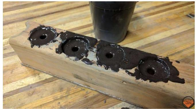
Attempt number 2! Instead of just a simple water/cement mixture I use epoxy and cement to give me a more solid mixture for turning and something that will be more stable when it's so thin.
