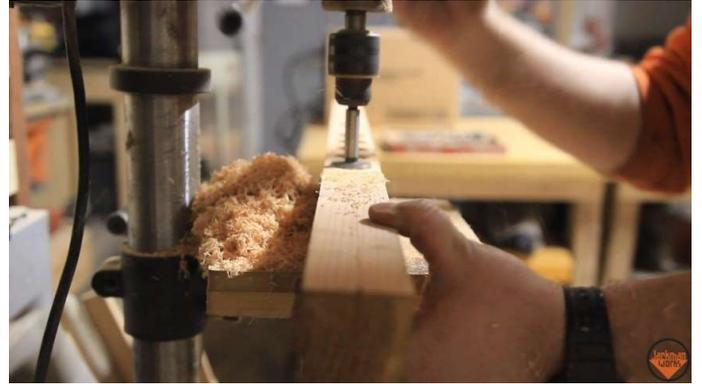
I use a forstner bit to drill out holes along the length of the wood form which will create cylindrical pours to make the pen from.
