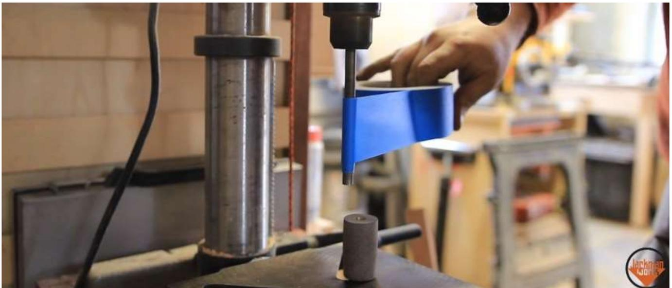
This project was part of a challenge to make a pen without using a lathe so I decided to utilize my drill press instead, figuring just about every woodshop has one of these. I mount a steel shaft in the chuck and pad it out to size with some tape until it fits super snug within the tube.
