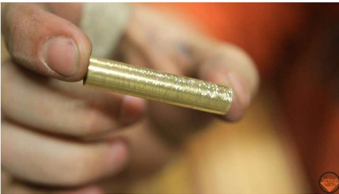
To help keep the tubes in place within the blanks I scratched the outside of them with sandpaper to roughen up the surface.
