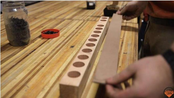
This piece of hardboard is used to cap the bottom of the form, it's fixed in place with a few screws.
