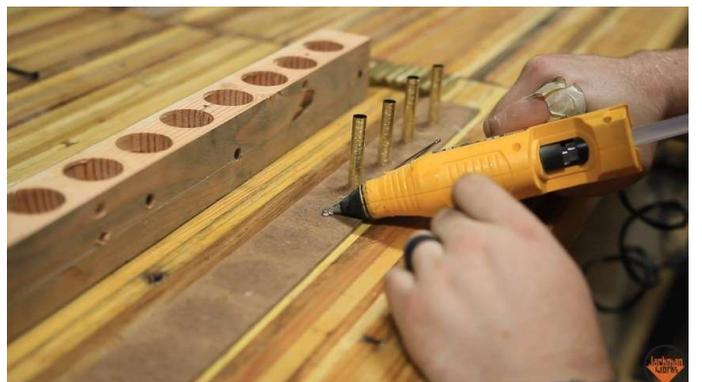
These are all stuck in place temporarily with hot glue. 12 tubes total which will give me 6 pens.
