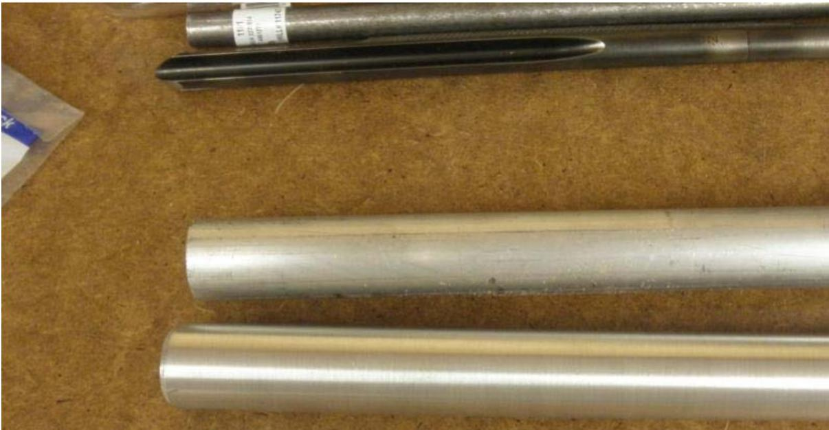
Not wanting any sharp edges, I used my oscillating belt sander and squared up the tubing. Then I put a 45 degree bevel on each end.
