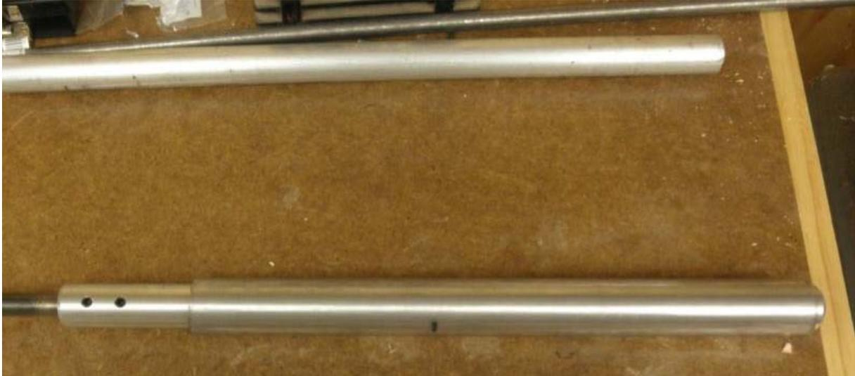
That's it for the 1/2" handles. Now on to the 3/8" detail gouge. Using the same aluminum tubing, I just had to make a little sleeve to fit the smaller diameter gouge. Fortunately, the 1/2" steel weldable tube fit the bill perfectly. It fit inside the aluminum handle and the gouge fit inside the steel. I also used 3/8" long set screws for this handle because I wanted them to make good contact with the gouge.
