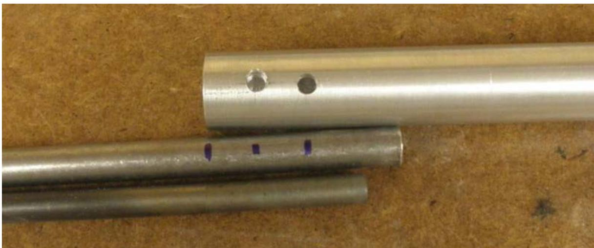
Then I drilled holes large enough to not cause any interference with the set screws. After I drilled the holes, I cut off the steel tube so it was just long enough to support the tang on the gouge (I just used the mark just to the left of the new holes).
