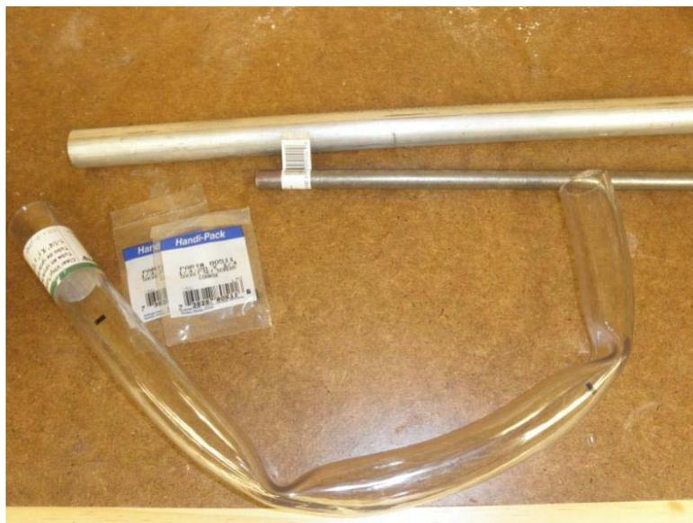
I got started by making handles for the 1/2" tools. First, I marked the tube with where I wanted to put the set screws. Then I used a center punch to mark the holes.
