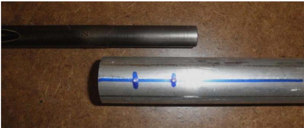
To drill the holes I used a small pilot hole and then changed the bit to 13/64".
