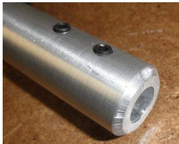
At this point I could have called it a finished tool handle but it felt a little small in my hand. I thought of options for making the handle bigger. Here are a few options: leather grip for an aluminum softball bat, friction tape for hockey sticks, or clear plastic tubing, etc. Obviously I chose the clear plastic tubing! It was a fairly tight fit but I managed to slide it on as far as I needed. Then I trimmed the excess with a sharp utility knife.
