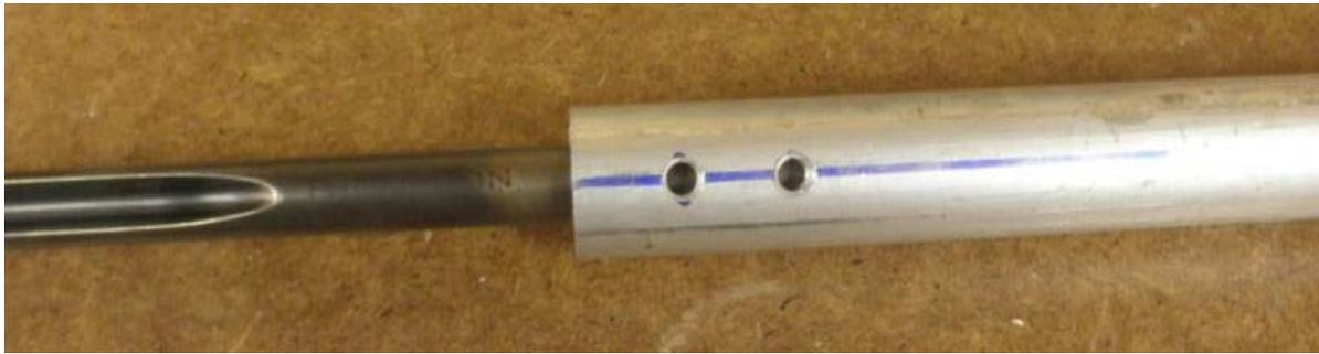
I could have left the aluminum as is but I wanted it to look nice. Using a chuck and a 60 degree live center I mounted the handle in my lathe and polished it up using sand paper. I used 150 grit and then just jumped up to 400 grit because I wasn't too concerned about a perfect finish. You can see how much nicer the finished handle looks in this picture.
