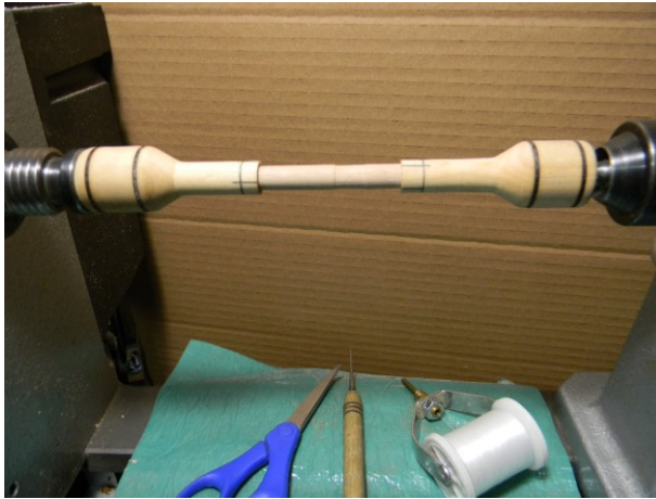
LATHE SET UP FOR WRAPPING THREADS
