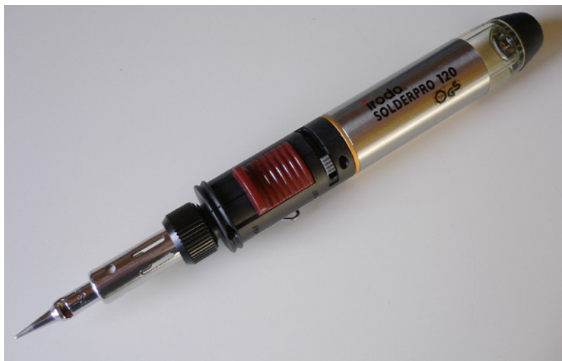
Iroda SolderPro 120 - Butane powered soldering iron/blow torch. It does struggle a little when its very cold as it is quite a small flame so doesn't cover a large enough area. Great for smaller joints and more intricate areas.
