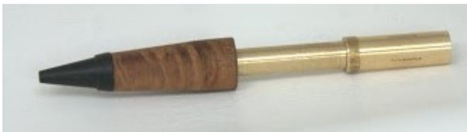
The next picture shows the 3 parts glued together with the 8mm tube and transmission coupler just slid into place I have done the final turning on the nose section yet. I use 3.200 inch (81.2mm) as the starting place for the length of the pen. That's measured from the tip of the nose cone to the back shoulder of the transmission coupler. This one ended up being 3.195 inch (81.1)
