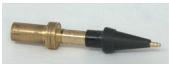
I turned the ebony for this piece to .400 inch (10.2mm) and then drill the different holes for the refill. I then turn the outer wall diameter to fit in the tube and cut it off. I then Mount it on the mandrel and turn the tapered shapes. I leave the largest diameter at .400 inch. This is not the finished diameter, that will be turned when it's assembled to the front nose cone and center band is turned as one.
