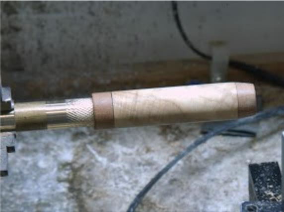
Because the mandrel is not accurate enough to turn the recess in the cap, I take it off the mandrel and wrap it in tape.
