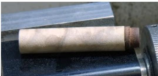
While its drying I make a brass mandrel to hold the upper body. I then mount the upper tube with the center band already glued on and turn it to size with the upper body. The upper cap is then glued on and the whole thing is slid onto the mandrel and turned to finished dimensions by file and by sanding.
