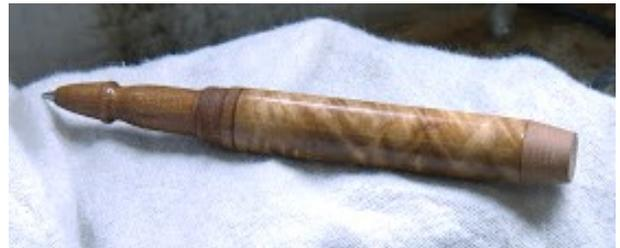
I then glue the cap in and mount the lower tube in the lathe using the blue tape. I sand and file it to shape and cut out the recess for the maple insert. The pen tube is already pre polished.
