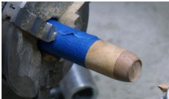
I use blue tape to protect the surface of the upper blank and mount it in the jaws of the chuck. I make sure that the seam of the tap is between the jaws, and I turn out the end of the cap for an insert of maple.
