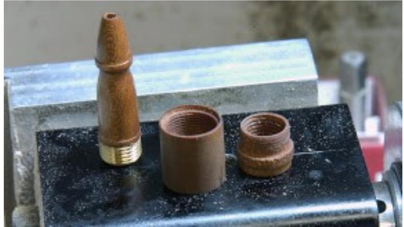
In the picture above, you see the nose cone with the brass sleeve with threads the center band and the nib coupler roughed out and threaded. The taps work great for the inside threads. The dies won't work I had to cut the outer threads on the coupler on the lathe by hand using a 60-degree tool and turning the lathe by hand. I have metal pieces that I have made that fit the threads cut in the wood to try them for fit.
