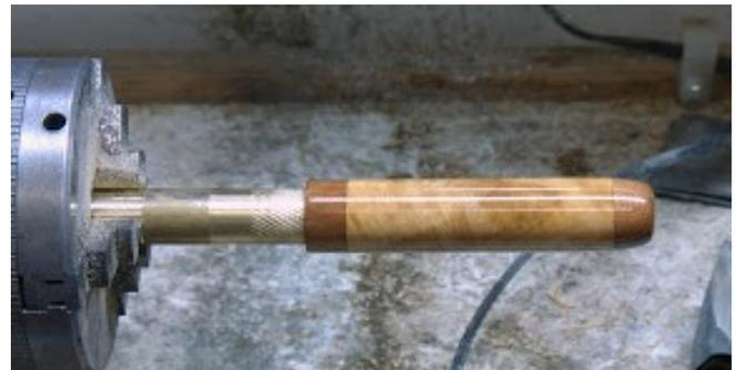
The next step is to finish the front tube. I make a mandrel for the front tube and turn the nib coupler and tube down together. Before I glue the top, I need to check the length of the refill in the pen. If I haven't measured right, I need to correct it now. I insert the refill all the way forward and the cap goes on easily.
