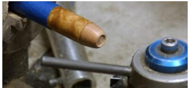
I cut the maple piece and glue it in and finish the pen. Because I'm using a friction polish, I peel the tape off the pen back to the jaws and blend the finish together. I then try the pen for fit. I used a small brush on a mandrel in the flex shaft with carnauba wax on it to polish the wood threads on the pen.
