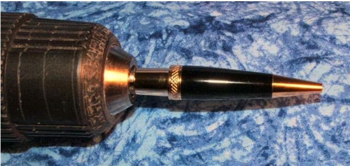
Recheck the fit of the insert into the nib end. (Note lettering)
