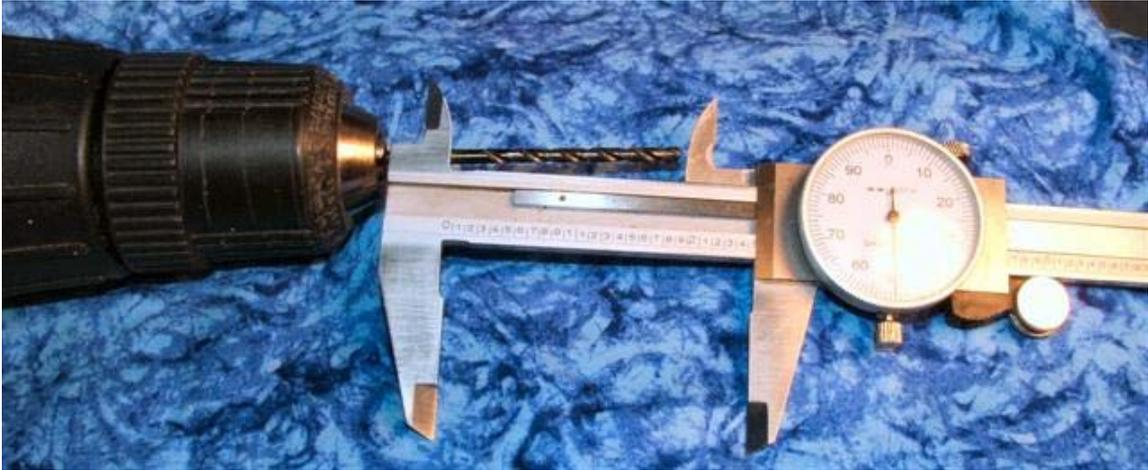
Now drill out nib end until the jaws or face of chuck bottom.
