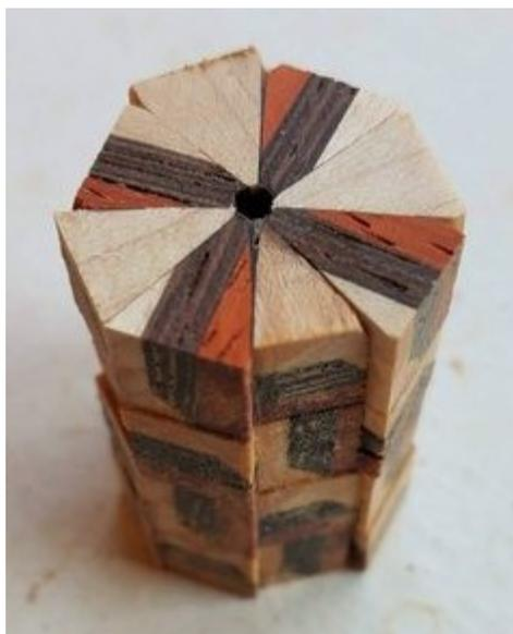
The hole is for a skewer to fit in to be able to center sacrificial end pieces for turning the blank round.
