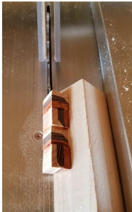
I then cut the other side using a 45 degree jig.
