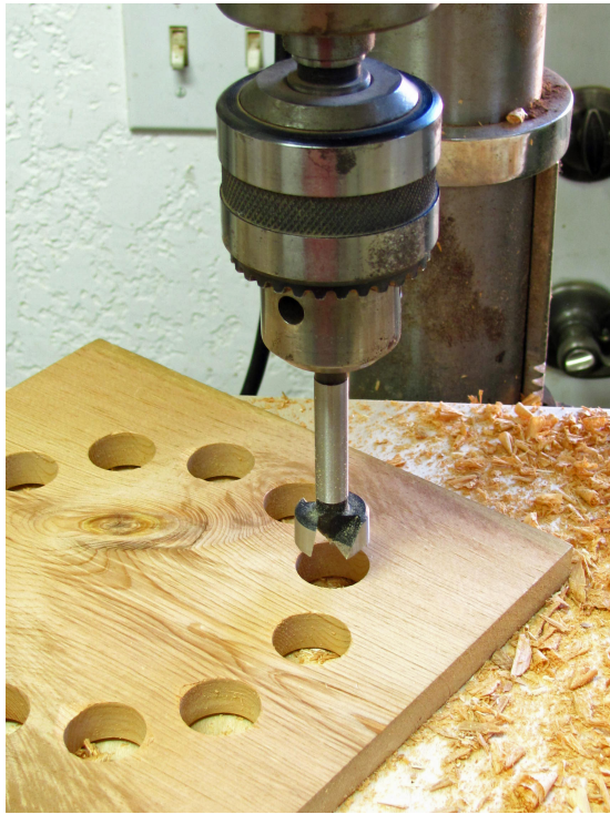
Drilling the \frac{3}{4} -inch holes in the top shelf.
