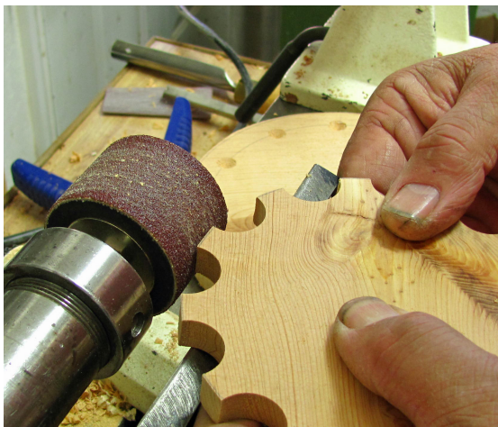
The 5-inch top shelf being tuned with a drum sander mounted on a mini lathe.
