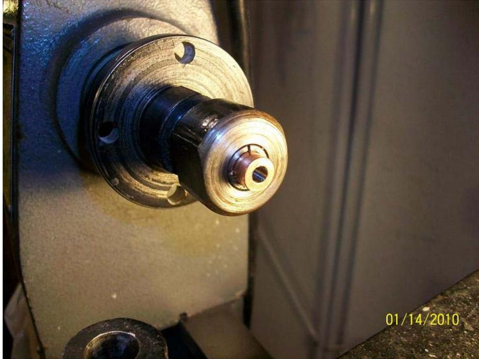
**Drilling complete, leave bullet mounted in chuck.**
