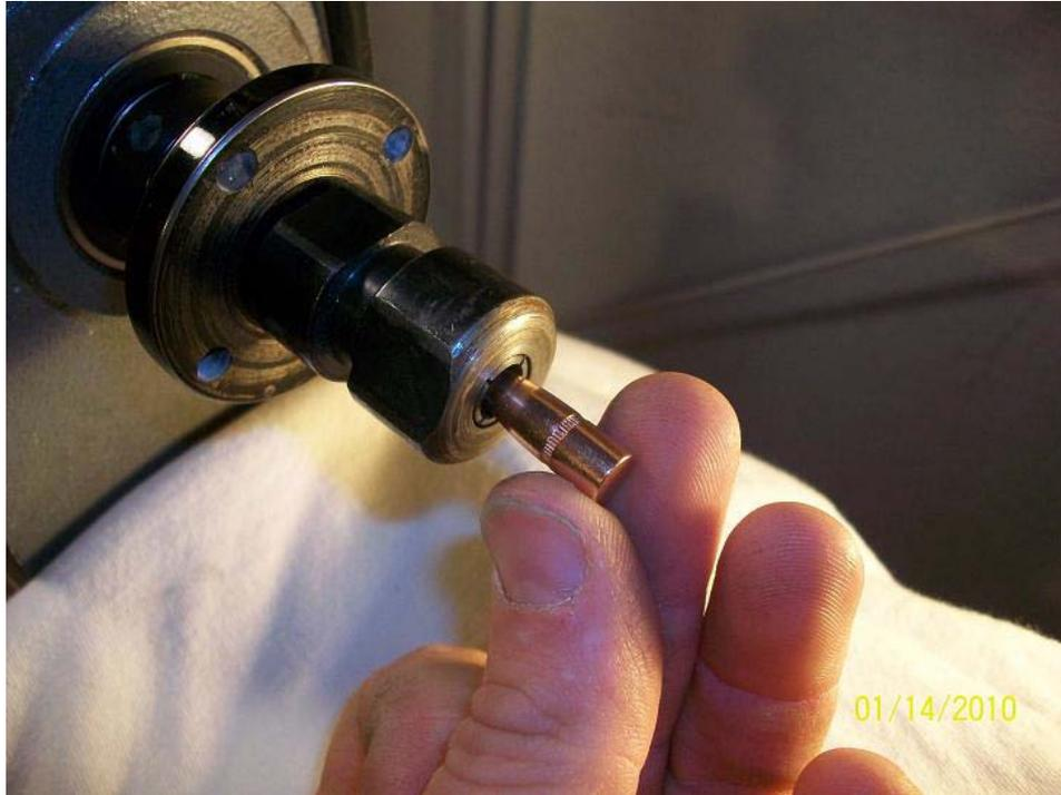
**Step 8: Insert bullet into chuck.**
