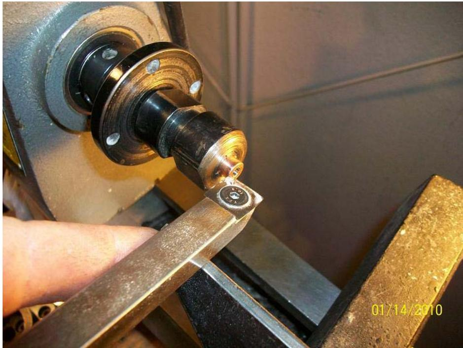
**Step 11: Create the tenon. I use the Easy Rougher for this step. The purpose of this step is to ensure that the brass tube, when inserted into**
