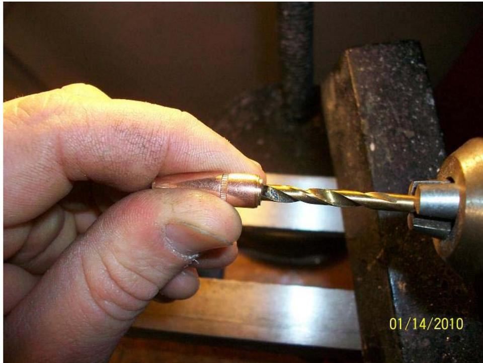
**Step 12: Test fit. Remove bullet from chuck and test fit the Cross ink to ensure a proper fit. You want the ink cartridge to stick out through the bullet tip a little farther than what looks normal. If it doesn't, push the bit through the end of the bullet as shown in this picture, and hand twist bullet to drill out a little more, then test fit again. Repeat step until desired depth is reached. Once this is complete, I will use 320 grit sandpaper and buff any rough spots smooth.**
