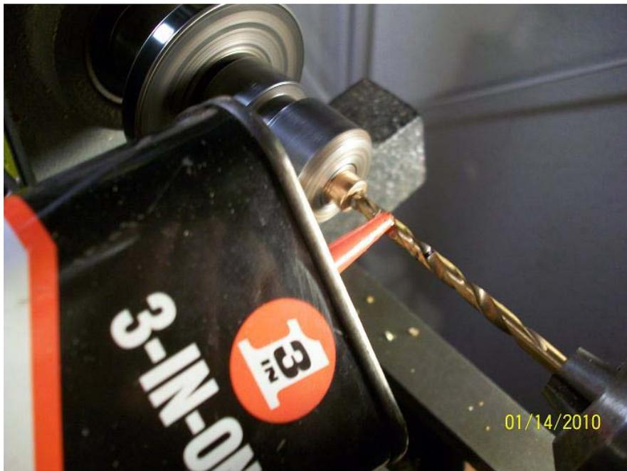
**Use some 3-in-one oil to keep drill bit cool. Again, keep your lathe on the slowest speed during this process. Continue to clear the lead waste as it is drilled by picking it off of the drill bit. I found that the more oil I used, the less locking up of the bit I get. If it does lock up, turn off lathe, and manually twist chuck in reverse (unlock tailstock) and back off the tailstock as you reverse twist the chuck.**
