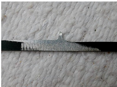
Close-up of single tooth on hacksaw blade. I started out with two teeth but took it down to just one and it seems to work better.
