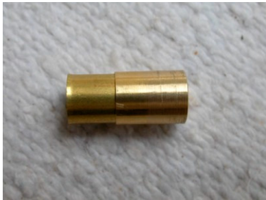
Above: Perfect fit transmission coupler/clip holder turned/sanded down to a "slip fit" so it can be pushed (not pressed) up through the tube to hold the clip in place.
