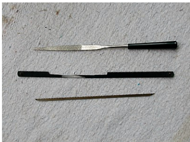
My current tools for recessing clips. Top to bottom: mini diamond file (HF), Mini hacksaw blade (ground away fore and aft, leaving one tooth to cut with), coping saw blade (ground away on ends for a small profile)
