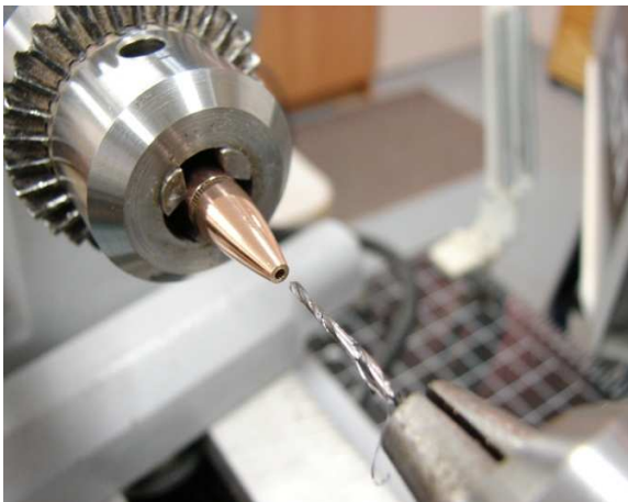
Drilling #55 Pilot Hole
