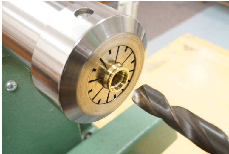
Countersink 21/64ths Hole to a depth of 5/64ths
