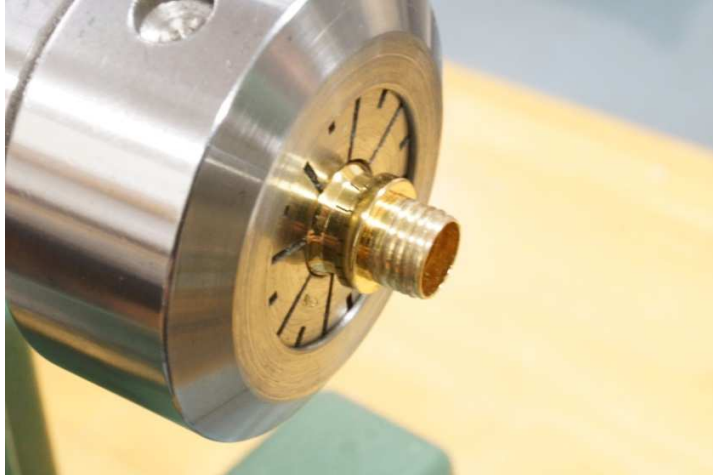
Bolt Chamber Threaded 3/8" – 24 UNF
