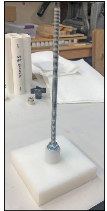
Figure 9. Assemble the Mold Base by attaching the Threaded Rod and 0.8" Straight Alignment Guide.
