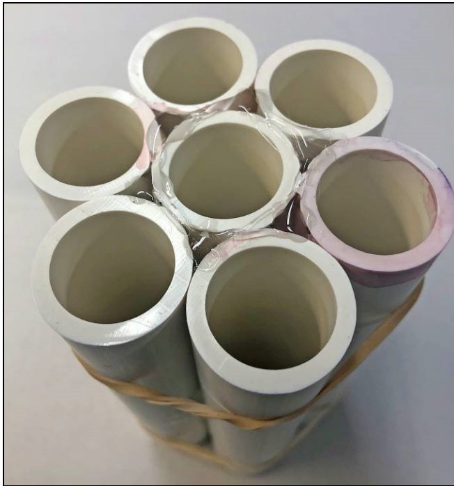
Figure 4. Hot Melt Glue pumped into spaces between the Pipes and the Assembly squared using a Miter Saw
