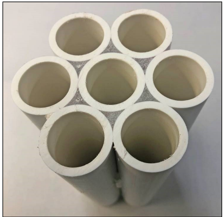
Figure 4. Hot Melt Glue pumped into spaces between the Pipes and the Assembly squared using a Miter Saw
