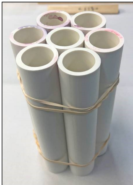
Figure 3. Seven pieces of Pipe held together with Rubber Bands and Glued together with Hot Melt Glue
