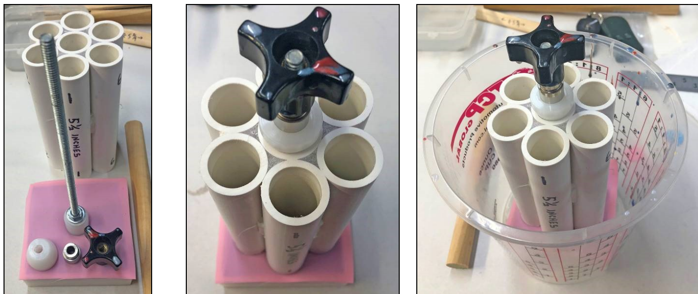
Figure 11. The Completed and Assembled Mold ready for use
