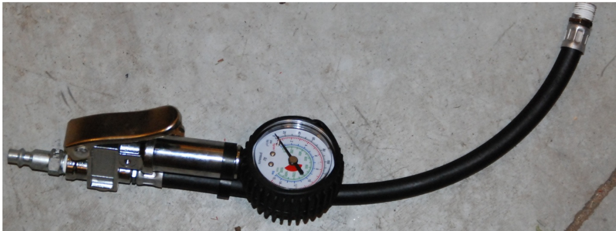
Figure 3: Harbor Freight's Dual Chuck Tire Inflator with Dial Gauge (Item #: 68271) with Quick Disconnect attached
