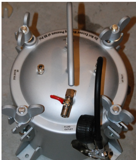
Figure 4: Completed pressure pot with tire inflator attached
