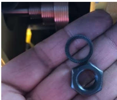
Figure 16. Jam Nut and Spring Washer
