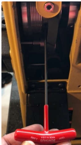
Figure 13. Spindle Pulley Set Screw Removal
