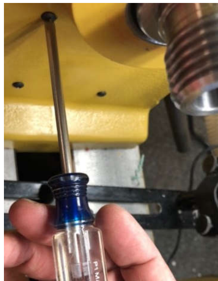
Figure 10. "Inverter Lower Box" Screw Removal
