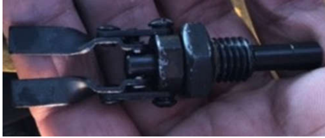
Figure 20. Spindle Lock Assembly
