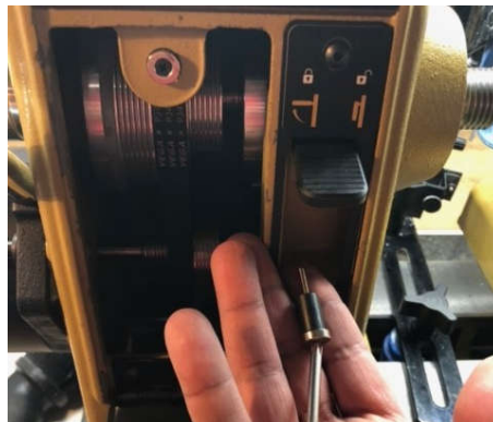
Figure 3. Magnetic Stop Removal
