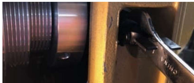
Figure 19. Nut removal using thin wrench
