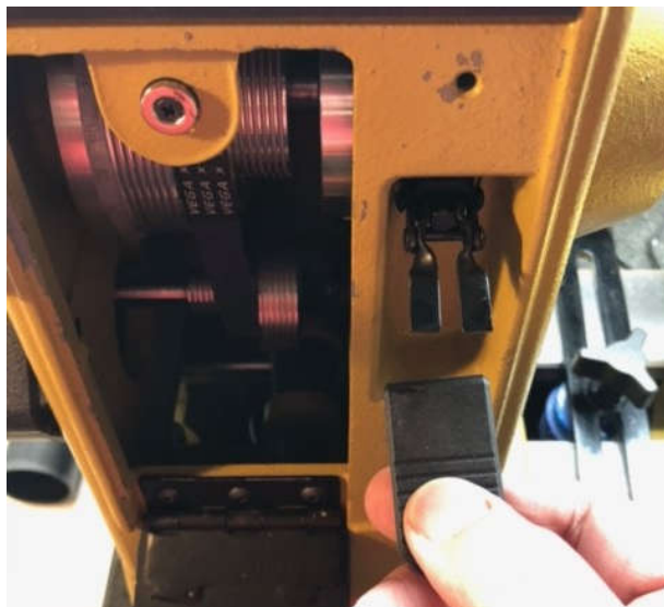
Figure 6. Spindle Lock Pad Removed
