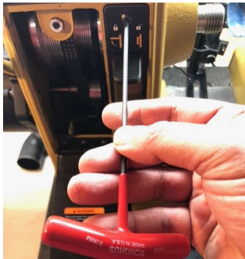
Figure 4. Spindle Lock Cover "Plate" Removal
