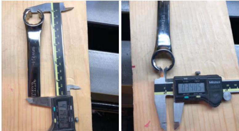
Figure 2. Custom 19mm, 12pt box wrench
