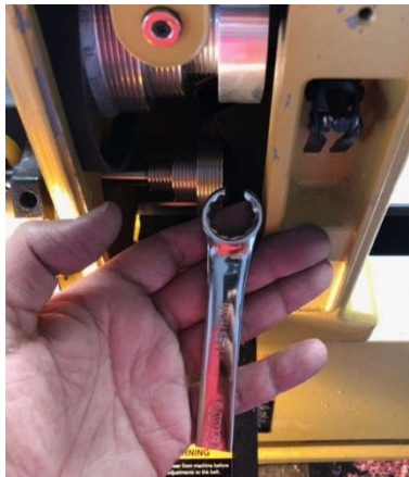
Figure 15. Spindle jam nut and spring washer removal
