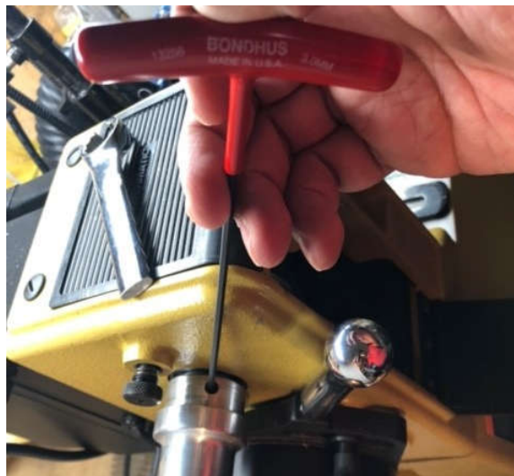
Figure 7. Hand Wheel Set Screw Removal
