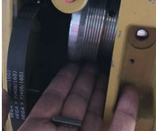
Figure 23. Spindle Pulley Key, long
