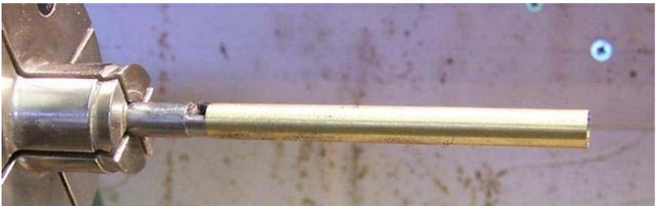
Here you can see why I didn't cut the threads off. I tapped an aluminium tube with the same thread (8mm) and made a handle for buffing. 🤖 As you can see, I am putting looooooong knurls on everything. (Thanks Joe Schmidbauer-jhs494 for the tips on how to do these.)
