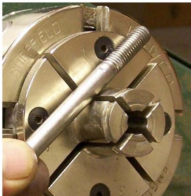
Put the bolt in the scroll chuck and bring up the tailstock. Note that I'm trying not to clamp on the threads. Select a distance from the end of the bolt approx. 3/4 of the length of the tube and make a mark on the bolt.
