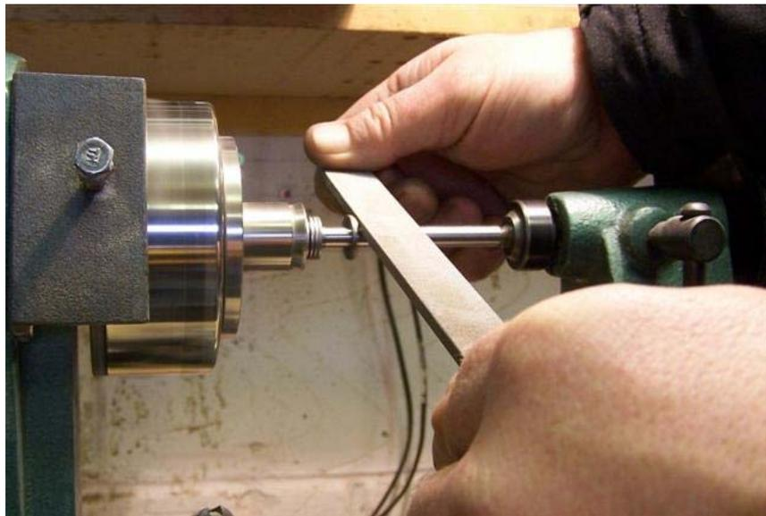
Once the caliper goes over the bolt throughout its length, you can remove the tailstock. Now change to about 240 grit wet'n'dry sandpaper and use it to get the brass tube to fit as snug as you can. Use the Sharpie pen to mark the high spots and start from the end.
