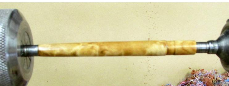
The blank is turned, sanded and a finish applied. Notice the recess on the right end for the clip. Take measurements from the original barrel. Also, did you notice I changed to standard slimline bushings and a mandrel? The longer blank was flexing being held between centers as the diameter reduced.
