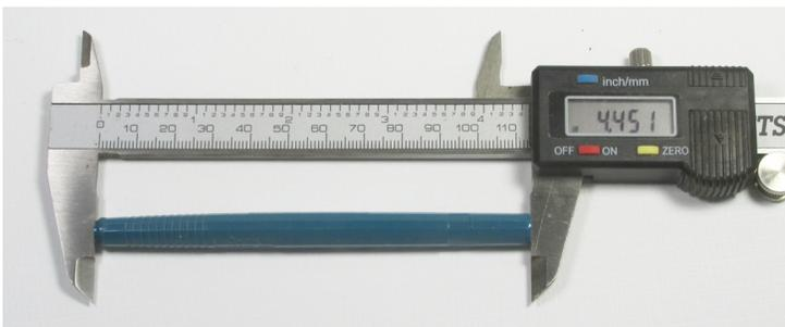
Measure the pencil barrel to determine the length of the new wooden, or plastic, barrel. The measurement is 4.451 inches. This is the length to cut the blank.
