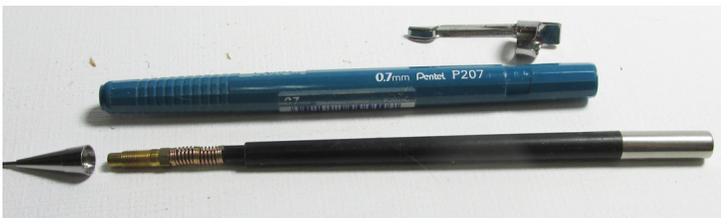
The writing tip will unscrew from the pencil mechanism and the mechanism can be removed. Remove the clip.
