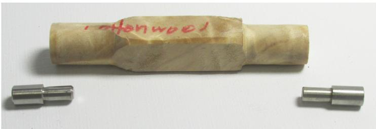
After the tubes are inserted square both ends tuning the blank to the correct length. I plan to turn the blank between centers using these two between center bushings holding the blank between a dead center and a live center.
