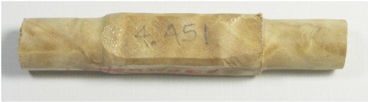
Longer bits, called aircraft bits, are readily available. Use a 17/64 aircraft bit first drilling totally through the blank. Then drill with a 7mm bit from both ends to enlarge the hole to 7mm.
