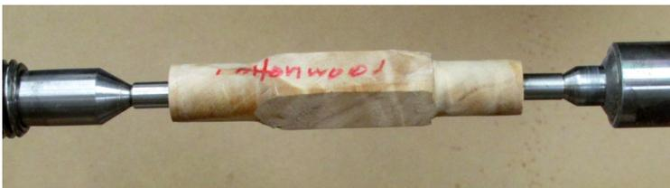
The blank is mounted with between center bushing between a dead center and live center.
