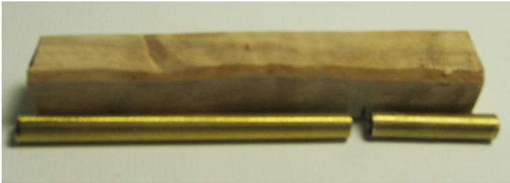
Longer 7mm tubes will be needed. 10" tubes are available. Two tubes will be needed: the longer tube is about 3.7" long and the shorter tube is the balance of the blank's length. The longer tube is glued in place flush with one end and the shorter tube is inserted in the other end. It is NOT glued in the blank.
