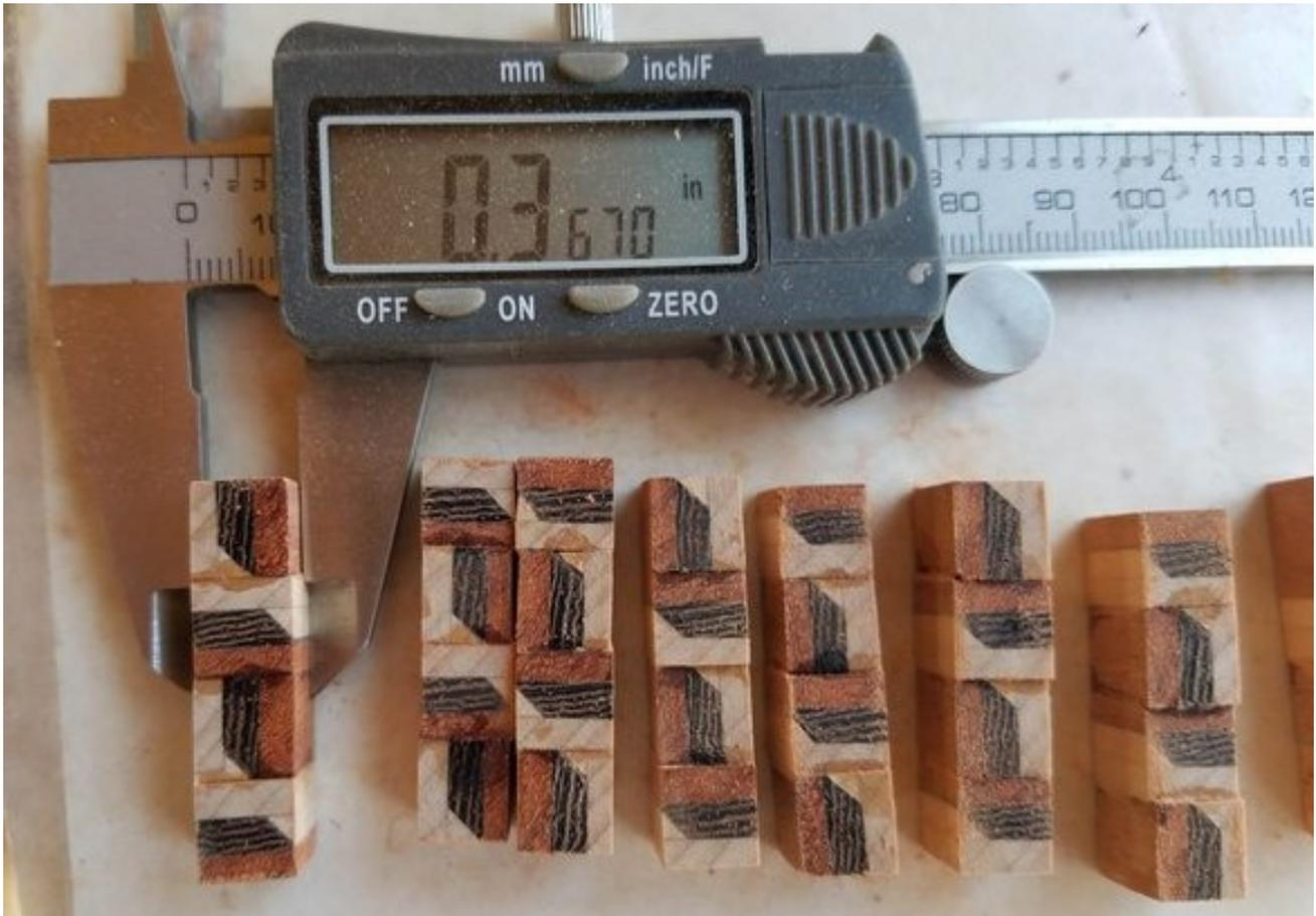
The next step is to saw these glued up pieces into staves. I used double sided tape on a 22.5-degree “fence” to cut the first side, then flipped the pieces over and repeated the process on a 45-degree fence.
