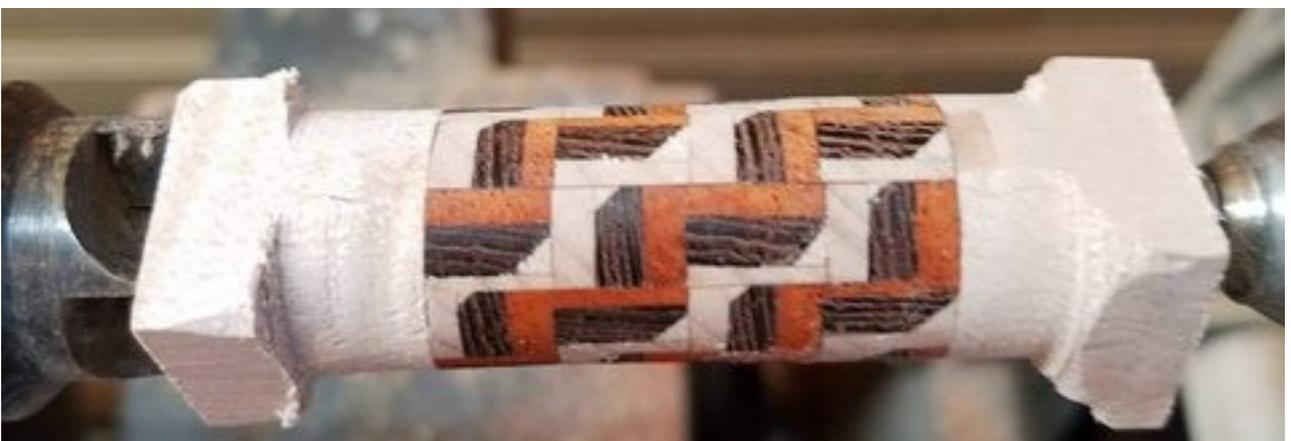
After replacing the maple end pieces with padauk, this is the final resulting pen. Note that on the unfinished piece above, the contrast is greater than on the finished pen. This is the result of using end grain instead of side grain.
