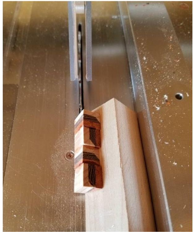
Then assemble and glue the staves into your barrel shape. Now remember to orient them correctly to carry the illusion around the blank.
