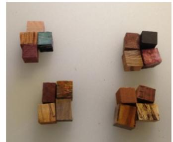
We now must glue the four pieces in each section together. Part of the charm of this pen is the lack of 90, 45, and 30 degree angles. To get this effect, I use my disc sander, and set the table at no more than 2 degrees off of square. Here I have set the table one degree off square. Here I am using an 80-grit disc which I have found to be of ideal to rapidly take off stock as needed and yet smooth enough to provide for a secure bond when gluing.
