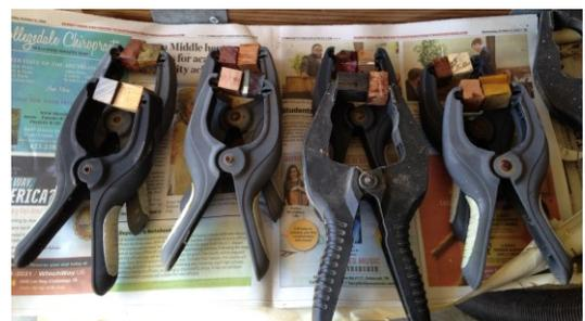
Next, sand the concave side of the glued-up doublets. You may have to sand one end of the doublet so that you have a stable base when you are sanding the concave side. Again, dry fit both halves of your four-piece sections to ensure they are flush, and when satisfied, glue together and clamp.
