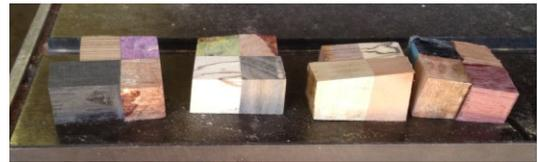
Next, dry fit in a stack, taking care to offset each section so as not to align the glue joints in adjacent sections. Turn the sections as necessary so that you end up with a somewhat vertical stack.
