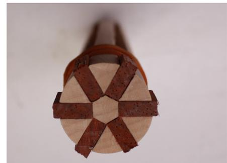
I knew the kit I wanted this for, so my tube length was also known. This is the rough draft for the design, and the final segmented inlays (shown just for reference for where I am heading). The dimensions can all be modified for the tube you may choose. The process is more important than the dimensions, but the rough draft is still helpful to determine the dimensions of each segment.
