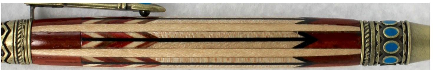
I decided to use a 75 degree angle for all the segments, and used a Spectraply pen blank for the feathers as I liked the color scheme. The blue tape was an easy temporary zero tolerance plate. I adjust my blade height frequently, and with the blue tape I can simple tear it off and have a perfect fit with a new piece. Slices were cut for the Chevron at about .077" width, for a final Chevron/arrow only of about .154". The angle and thickness are all adaptable.
