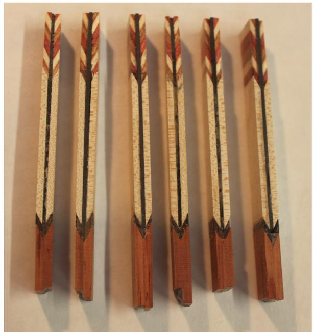
A test fit, and the glue-up with 2 part epoxy.
