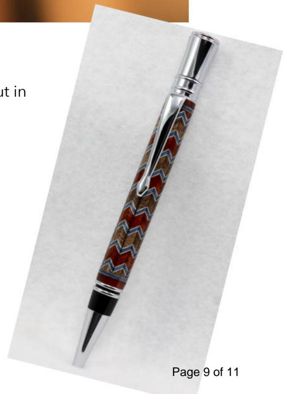
As mentioned earlier the thicknesses of the chevron slices were important to eliminate the material between the Chevrons but extending to the OD of the finished pen. I did experiment with several methods, but ultimately decided on the "star" shaped hexagonal design.
