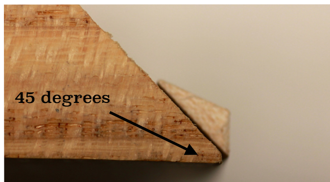
Sanding the 45 degree angle
