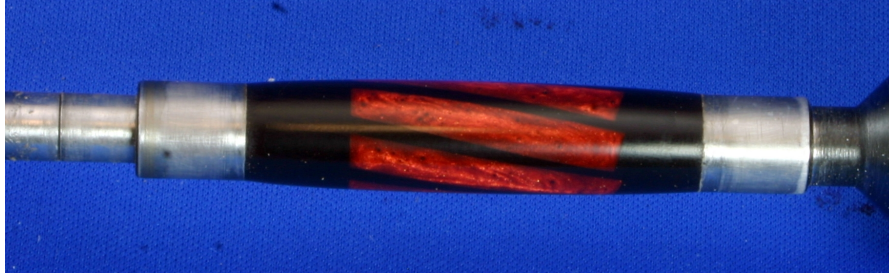
Figure 9: All voids filled. The blank has been turned and sanded.
