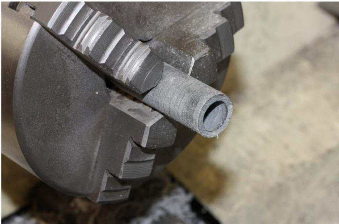
Then drill for the tap used, in this case M12x0.8, I use 7/16" for this, but 11mm can also be used if a slightly skinnier section than the El Grande is used.
