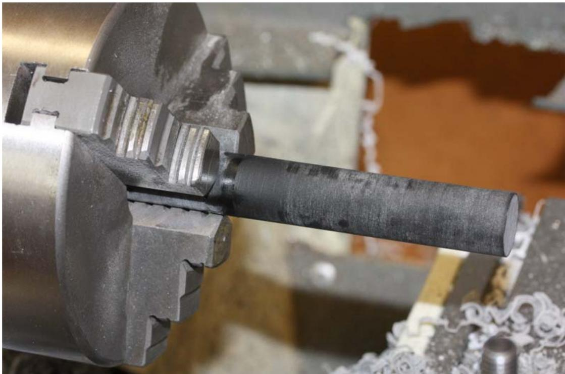
When all this is done the cap should screw on the barrel neatly, which it does!
