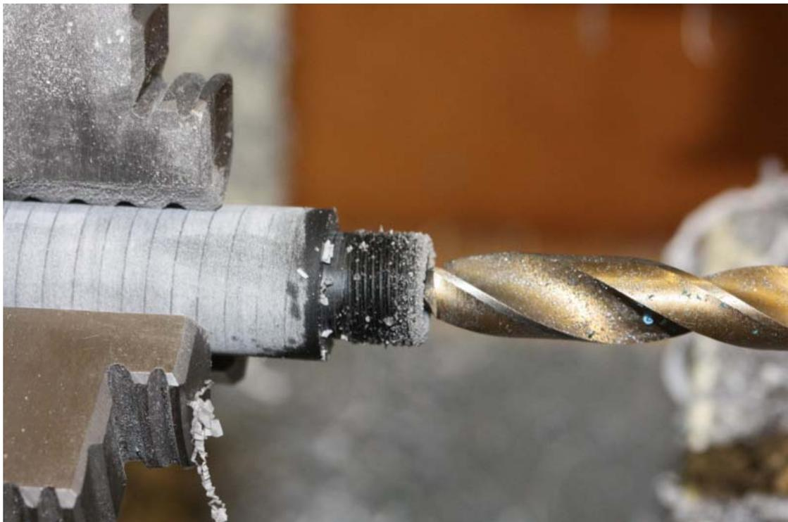
The hole is then drilled out to 9mm (M10-1) to the same depth.
