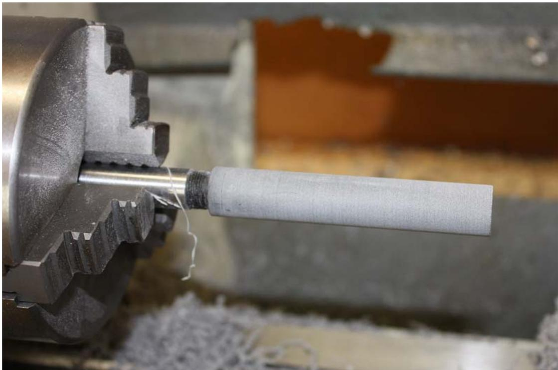
Turned to intermediate size ready for finishing on the wood lathe, using the same closed end mandrel in a collet chuck
