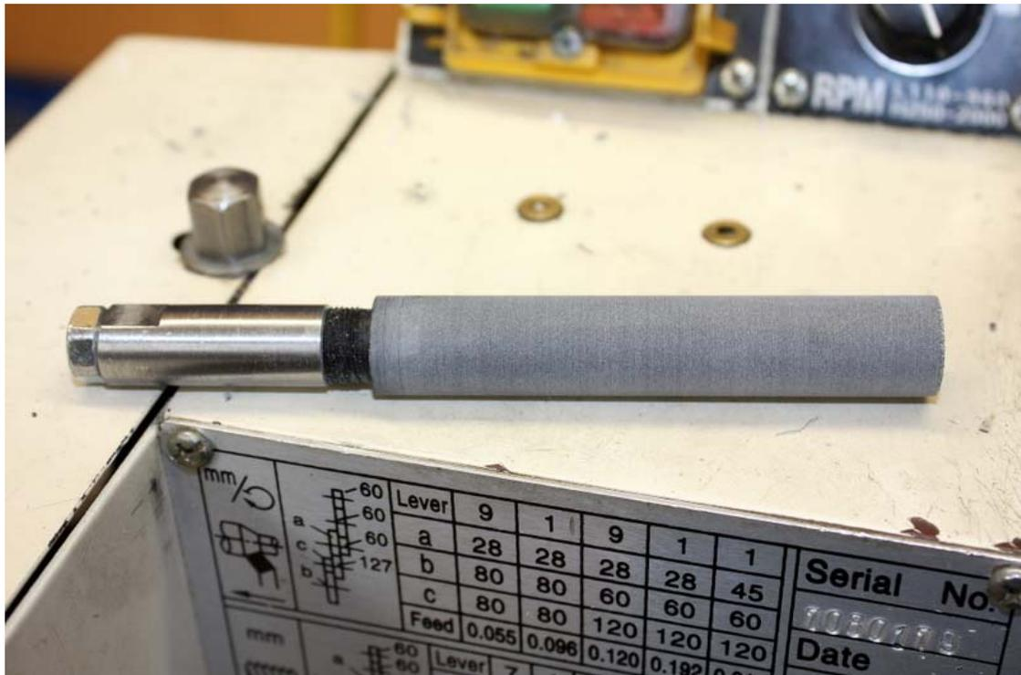
The cap still needs a finial and clip, drill for an M10x1mm tap, then turn a finial with a tenon and thread with an M10x1mm die
