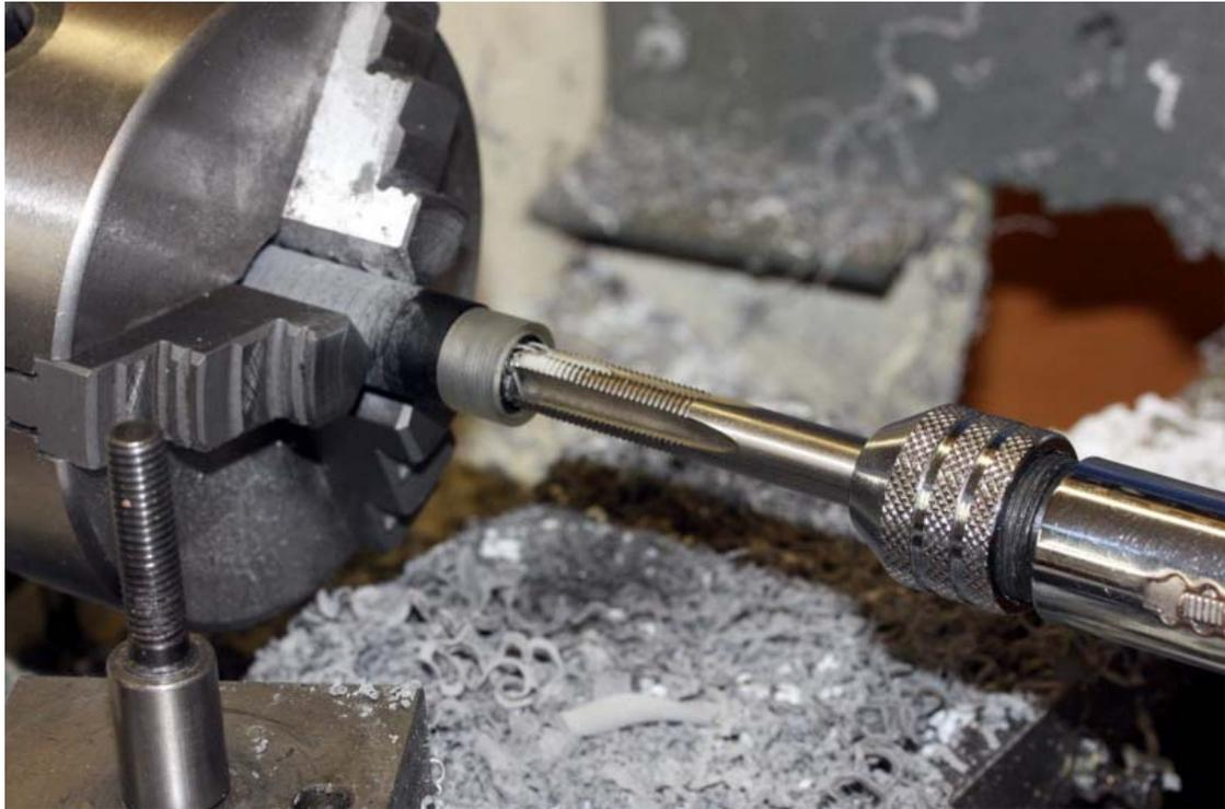
Again making sure to use the canola cooking oil as a lubricant, cut the internal M10x1.0 thread to at least the depth of the thread on the section.
