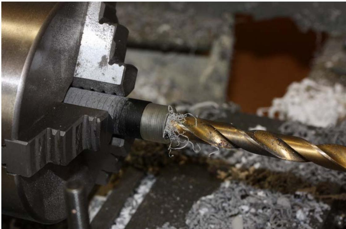
As the thread on the section doesn't run all the way to the shoulder, the internal thread is undercut to allow for this, using a 10mm drill.
