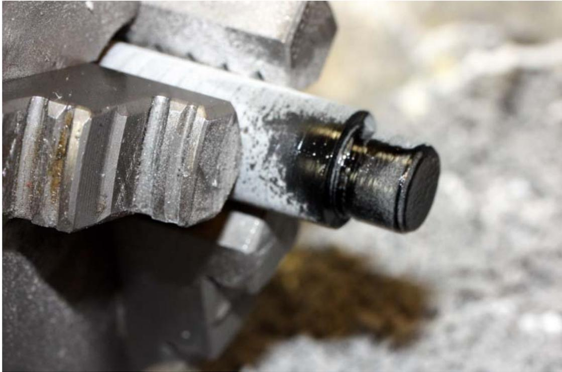
It is very important to use a lubricant when threading most materials, particularly on Polyester resin (PR).
