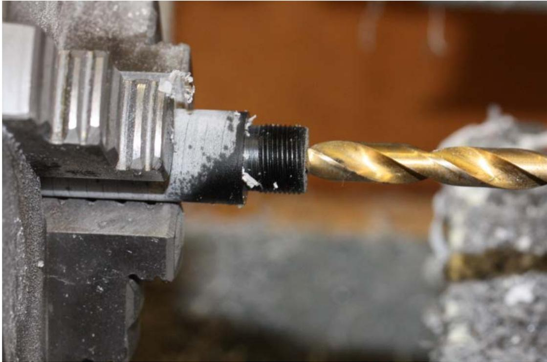
After centre drilling, a 7mm drill is used to drill a starter hole, about 70mm deep, this can vary with the type of and length of pump or cartridge.
