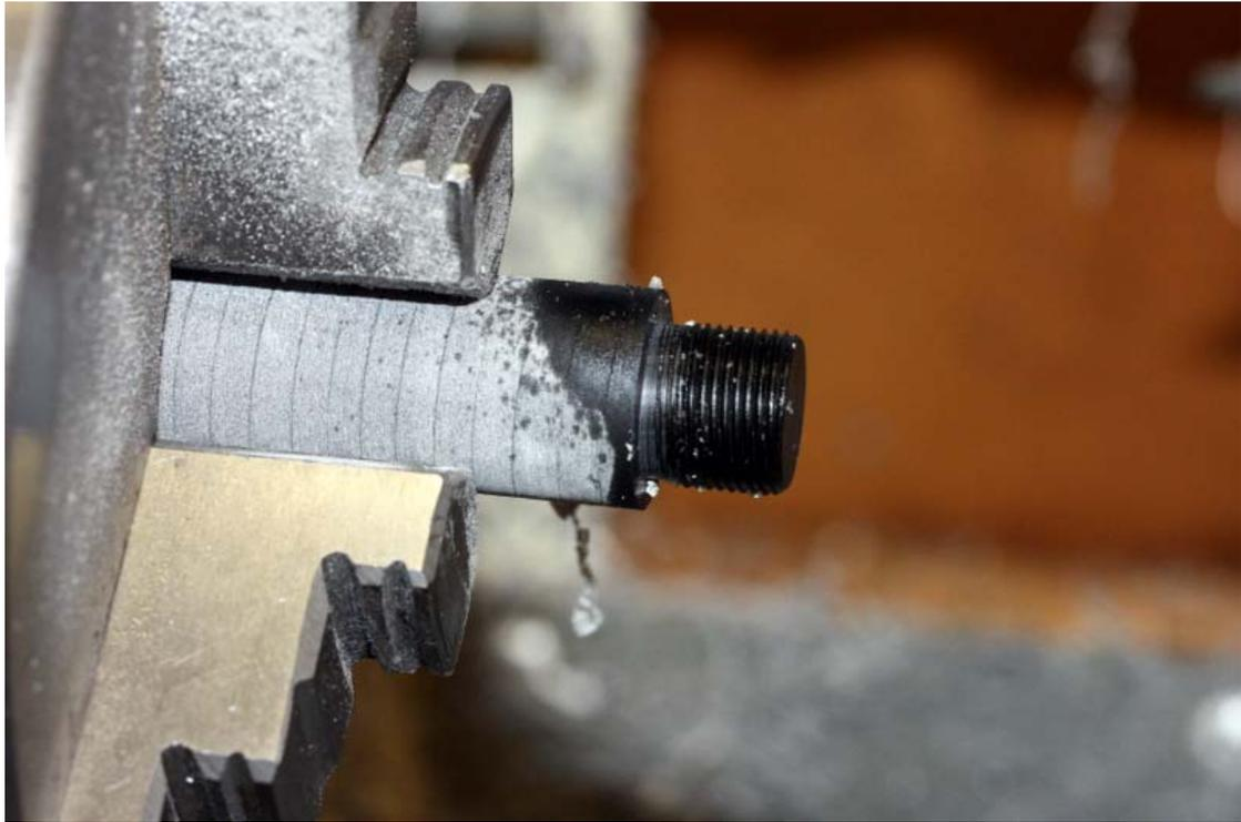
Once the whole thread is cut, the die is reversed in the die holder and the thread re-cut right up to the shoulder.
