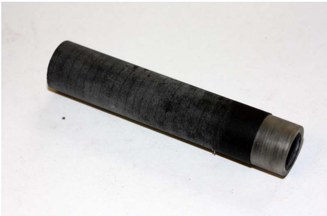
The barrel is now ready for final turning to the required shape. I use a closed end mandrel for this, similar operation to making a closed end pen.
