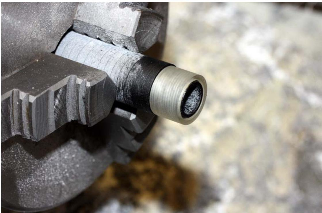
To assist with threading and minimise the risk of breaking I use a clear PR collar pre-threaded to the thread used on the OD (see separate tutorial).
