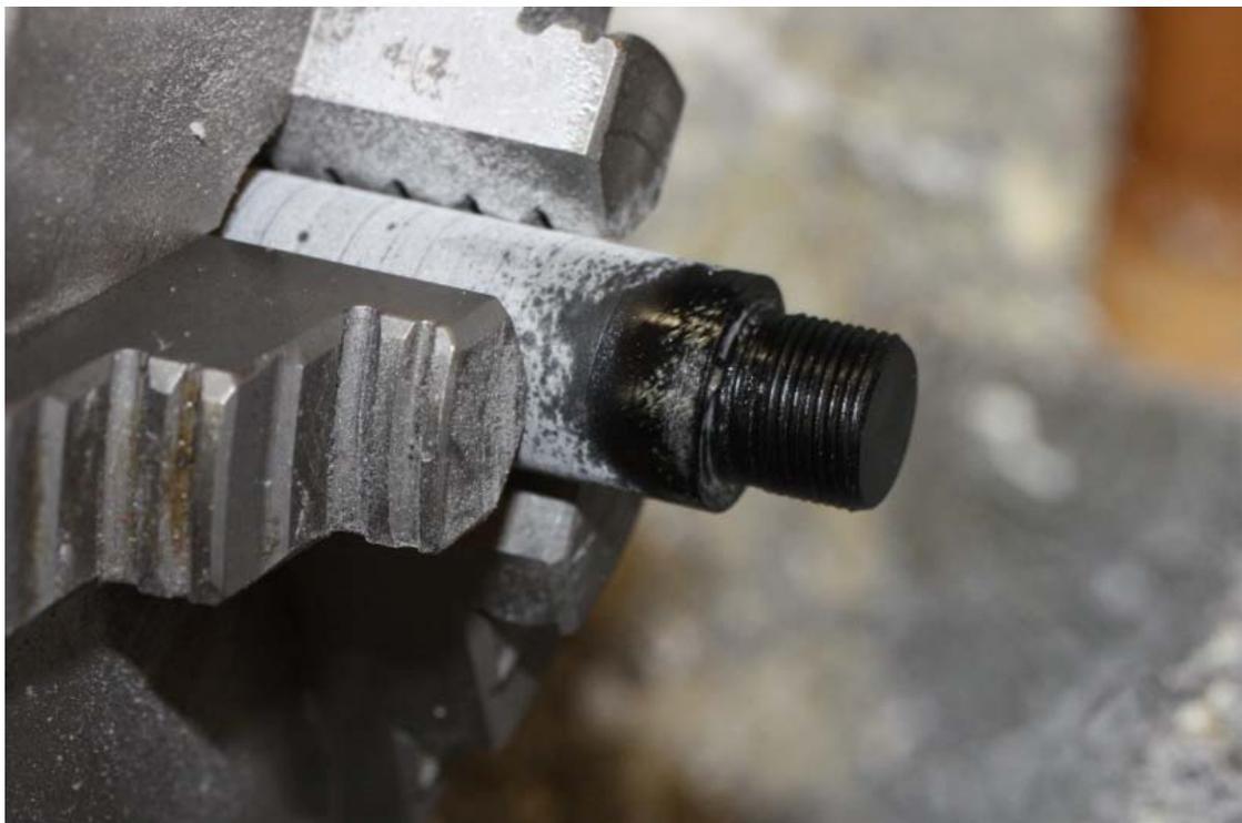
The thread is cut with the M12x0.8 die mounted with the size information facing the blank. Only cut small turns each time, then reverse a bit and keep swarf out of the cutting area. I use compressed air here.
