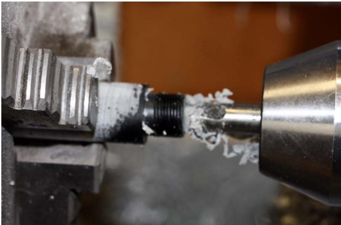
Now we can start on internal thread which will take the section. In this case I am using an El Grande section which is threaded with M10x1.0.
