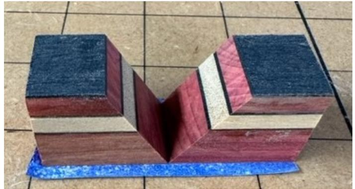
Cut a piece of tape and lay those two little pieces next to each other on the tape. That tape is now a hinge and will perfectly align the pieces. Put a little CA in there and close them together. Try to keep CA out of the center; you want a nice sharp point in there.
