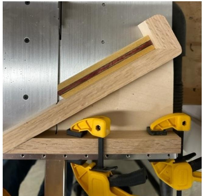
Rotate the blank 180 degrees and make the same cut. The point will automatically be centered on the blank.
