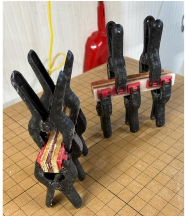
Unclamp and clean up the blank, making sure the blank is square!!
