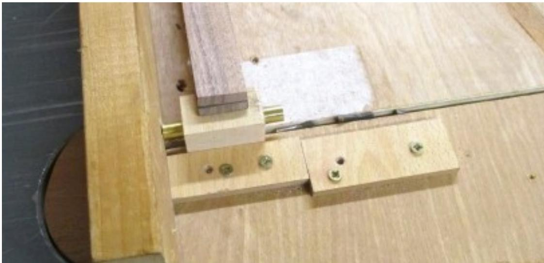
The purfling is epoxied into the slots created. When the Epoxy is cured, I trim the blank flush with the purfling and then I'm ready to add ends and turn to finish the blank.
