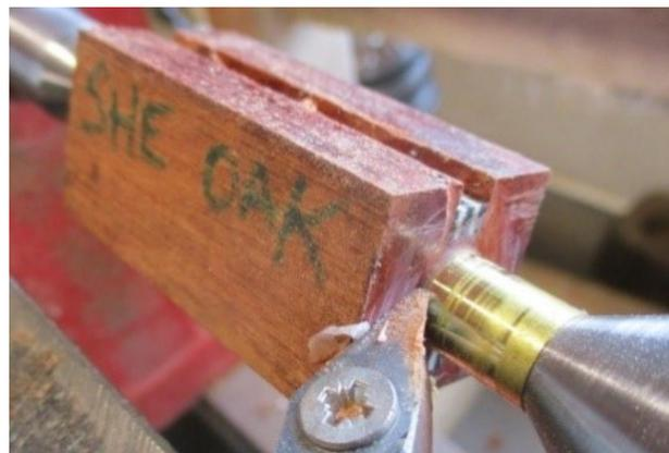
Below you can see I'm using brass rings to determine the final cut depth to gauge how much purfling is left after finishing.
