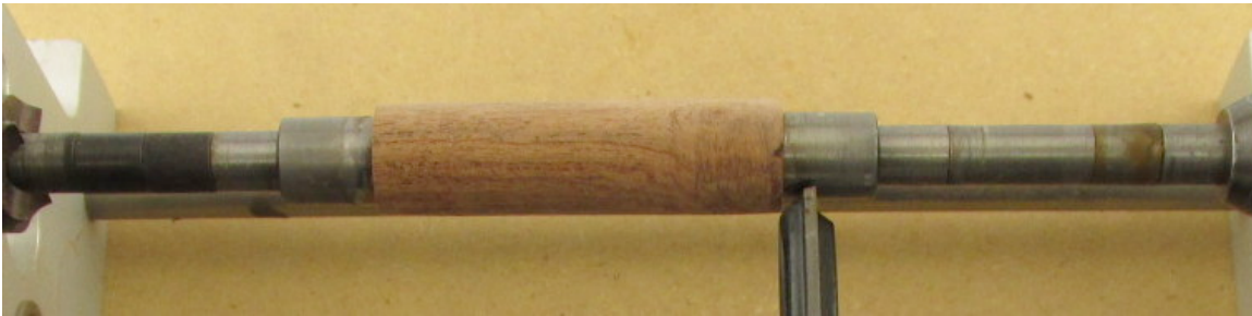
Figure 8: The blank locked in place on the mandrel and the cutter in position.
