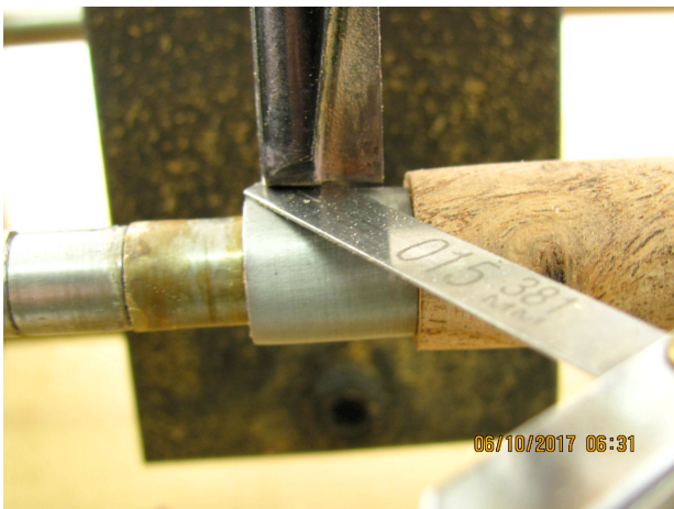
Figure 9: The cutter positioned using a feeler gauge.
