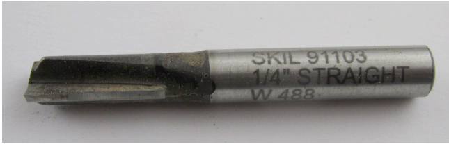
Figure 7: The straight cutter used for the hexagonal barrel.
