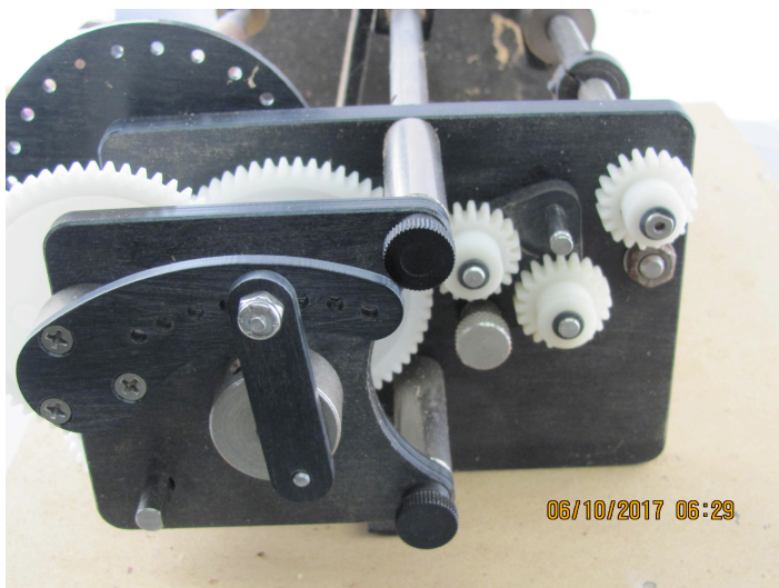
Figure 11: The gear connecting the lead screw gear to the others is removed and the mandrel gear in neutral.
