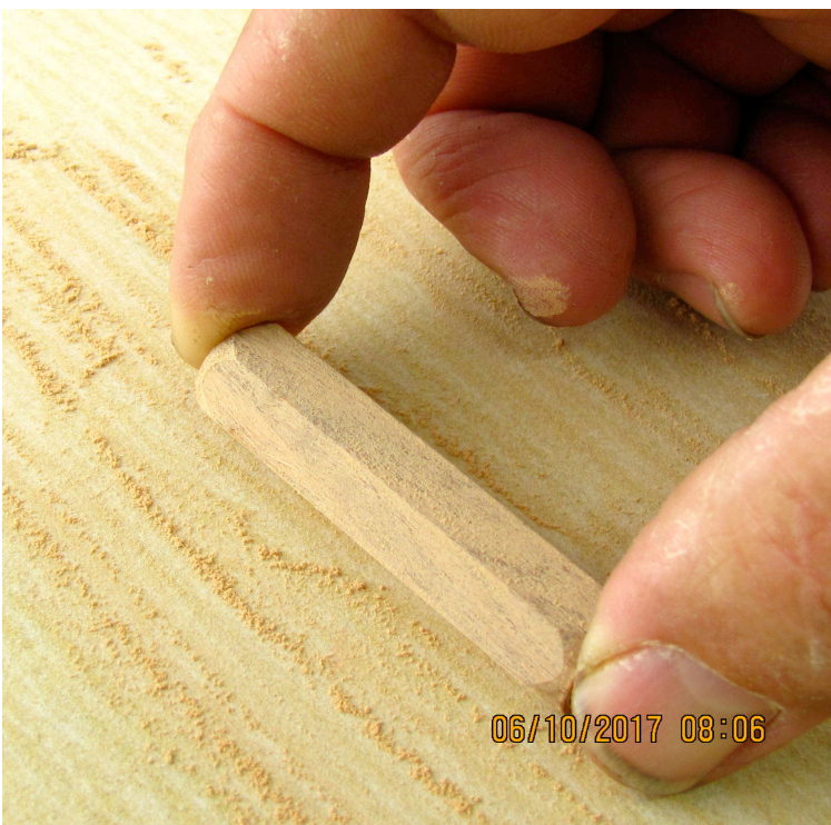
Figure 16: Sanding the flat sides of the hexagonal pen barrel.
