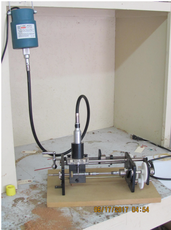
Figure 5: The Harbor Freight Flexible Shaft Grinder/Carver attached to the Pen Wizard.
