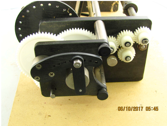
Figure 10: The gearbox and Guilloche attachment.
