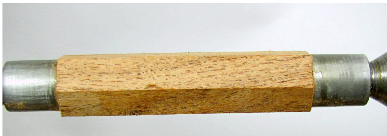
Figure 14: The blank after making 6 passes for the hexagonal pen barrel.
