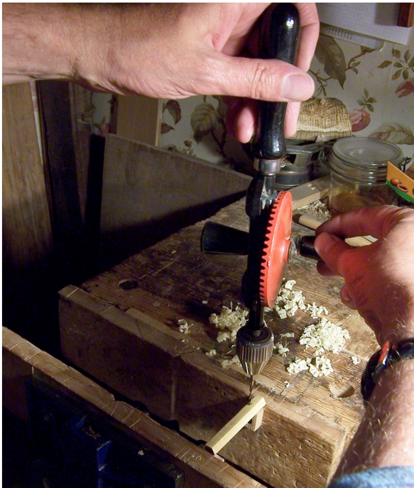
Figure 31: Using a hand drill to make hole for the mother of pearl dots.
