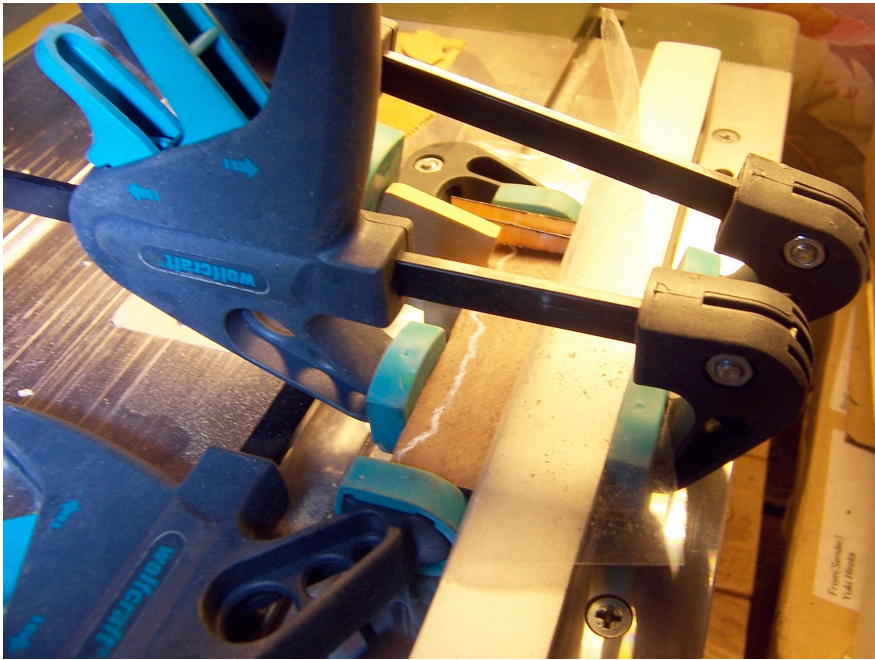
Figure 22: Gluing the white veneer strip in place.
