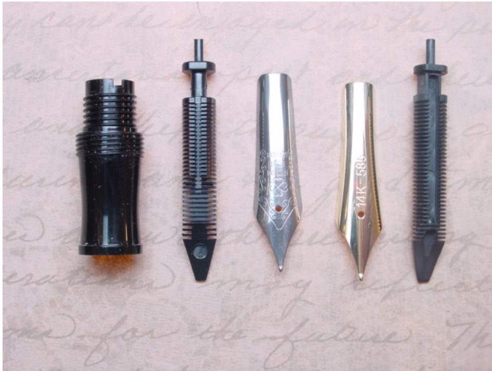
Ligero front section, stock feed & steel nib, replacement 14K gold Penchetta nib.
