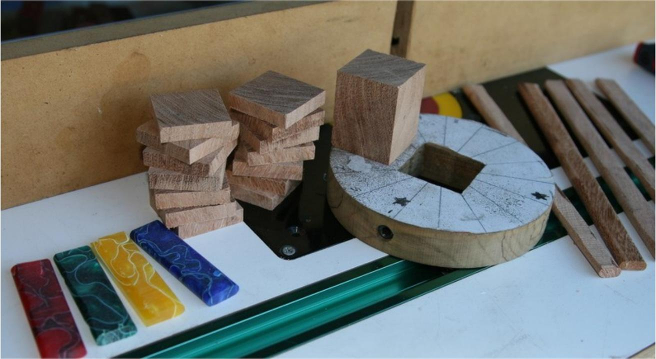
When you are ready to make the first cut, draw an arrow on your blank, the part of the blank you have left over after cutting the 1/4" squares off and point it to the #1 position on the indexing circle. Every time you put the blank back in the indexing circle, the arrow should always point to the #1 position. The first cut will be on level 1, so start with #1, on the indexing circle going into the router first.
