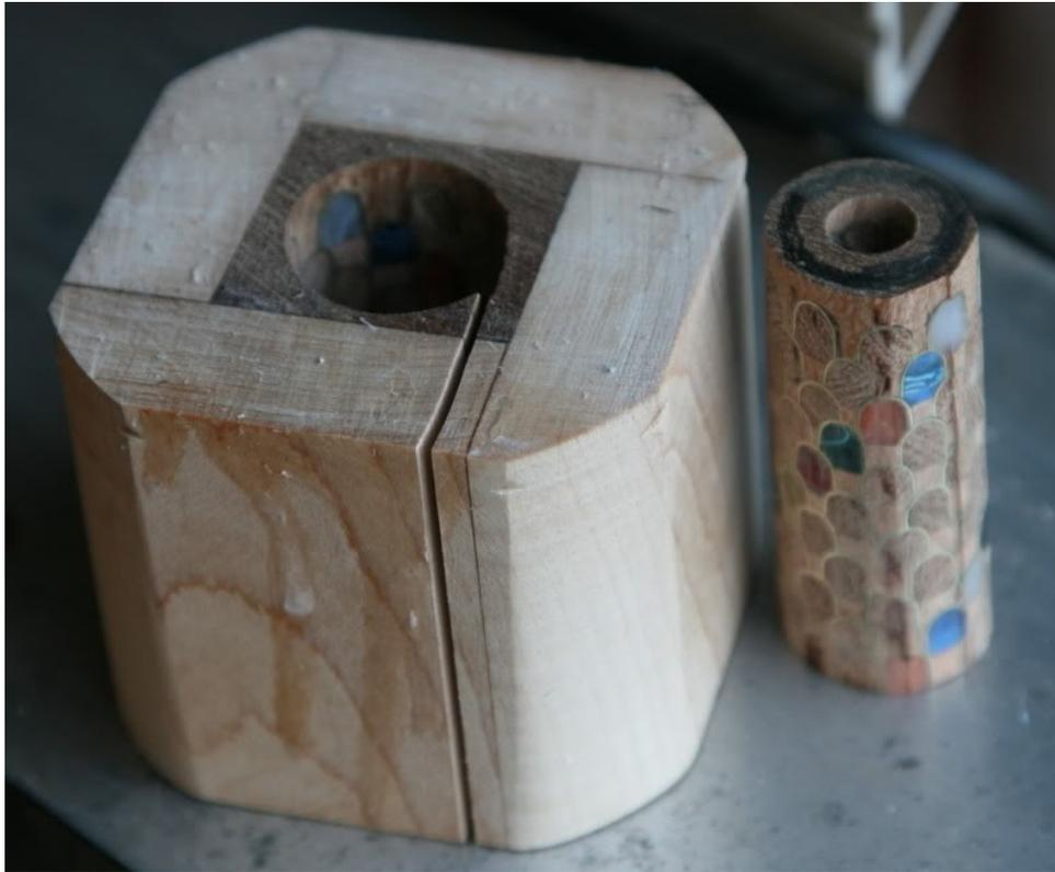
No matter how sharp you think you have your gouge or skew, the second it hits any kind of metal, the sharpness is history. From this point, only use sandpaper. Start with 80 grit and go all the way through 600 grit. Then use MM, WET sanding all the way through 12K. Wet sanding will clean out all the dust and polish the brass or any other metal you are using. YES, it will take little longer, but in the end, you will have a beautiful pen and not need to start all over again.
