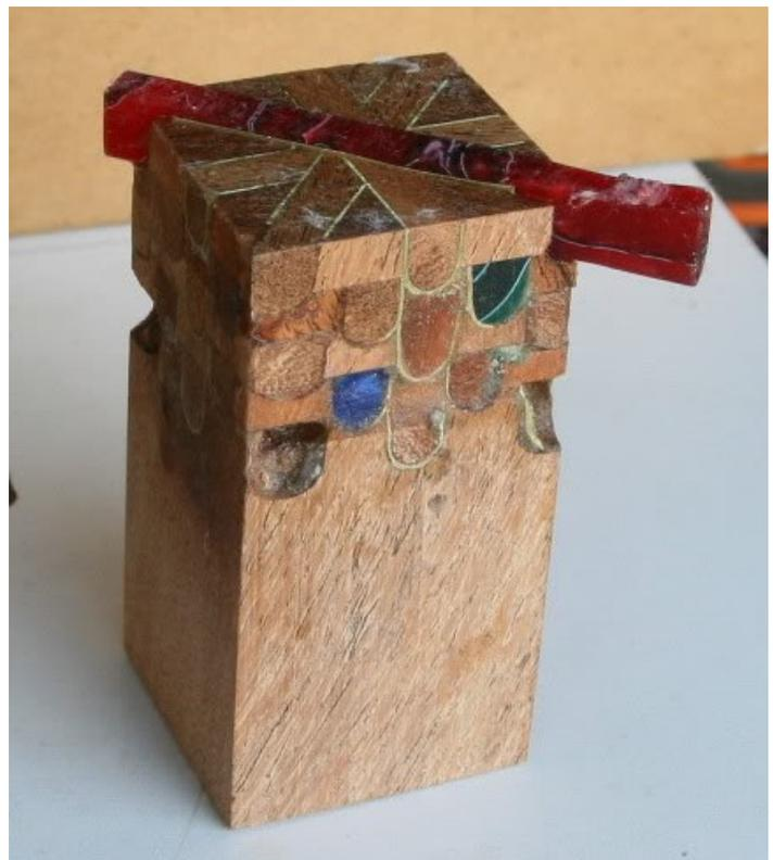
After you have glued a piece of brass and wood into the first routed section and let it "dry" sand the excess down so the blank stays square.
