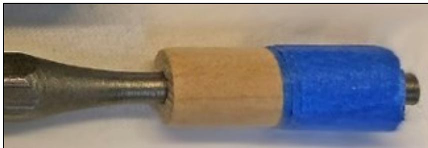
The old \frac{3}{8} " wooden Punch Guide (Pictured on the Punch)
