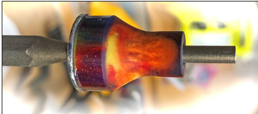
The new, more robust metal and plastic Punch Guide (Pictured on the punch)
