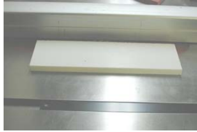
Corian used to set blade Height
