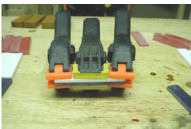
Strips glued & Clamped
