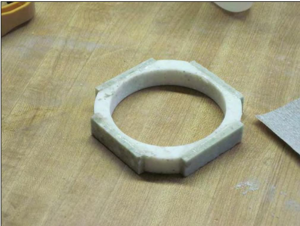
11. Cut the blank again on the table saw, this time with the miter gauge set to 45. Then glue your second color on.
