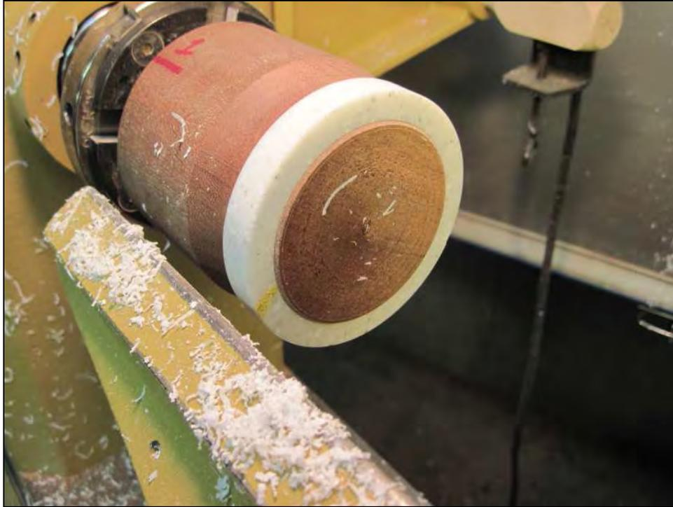
8. The blank is then cut in preparation for insertion of an embellishment that adds a segmented quality to the bracelet:
