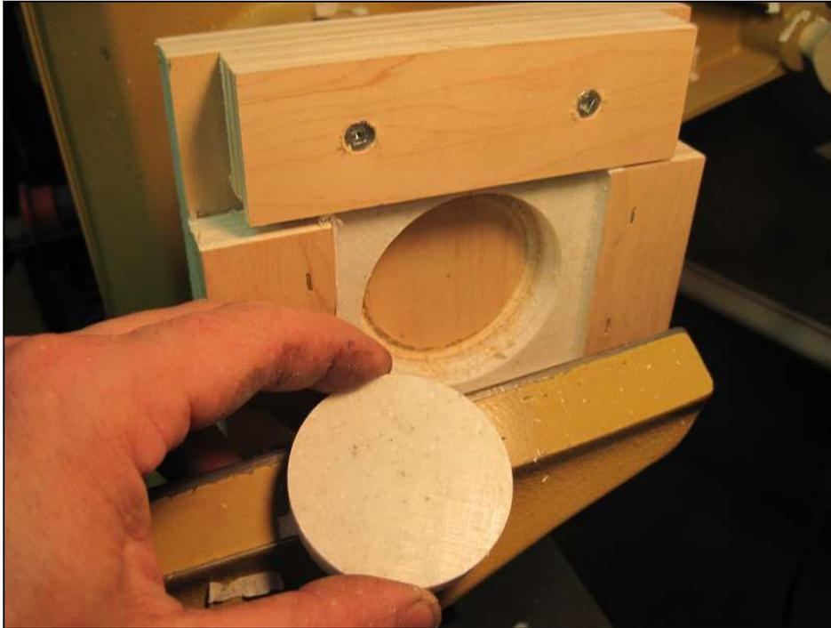
4. The blank is routed to the desired diameter using a jig made on the lathe.
