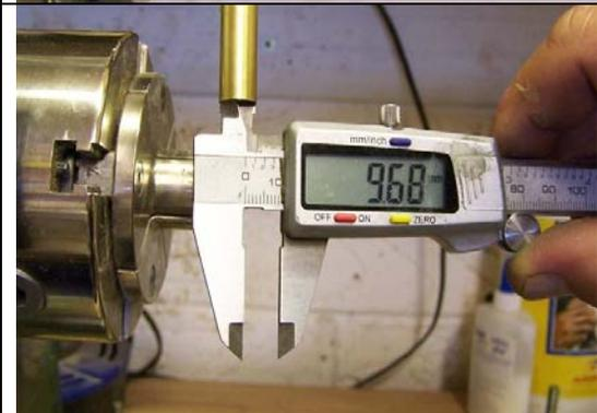
pic 5; Measure the inside of the tube
