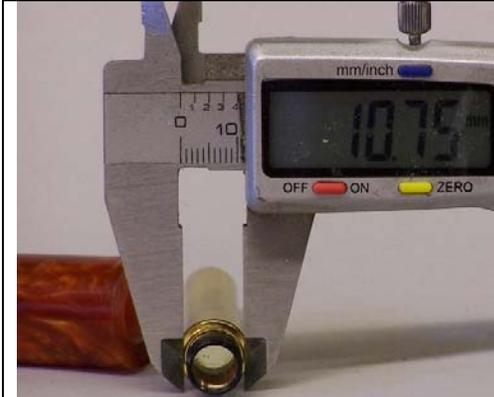
pic 14; measure the dia of the inner ring surface
