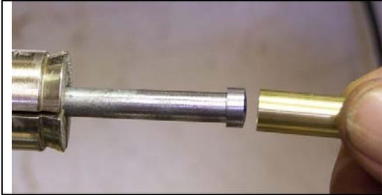
pic 6; the end filed down to match the tube ID
