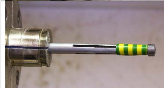
pic 9; a layer of tape should easily hold all jaws together if the slots are long enough
