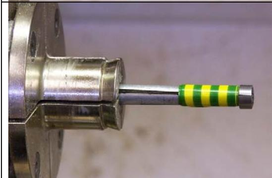
pic 10; move it deeper into the chuck
