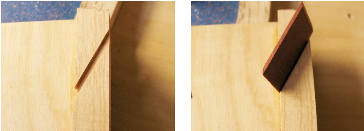
Figure 3 - Left: Saw Blade cut groove in bottom of Hold-down
