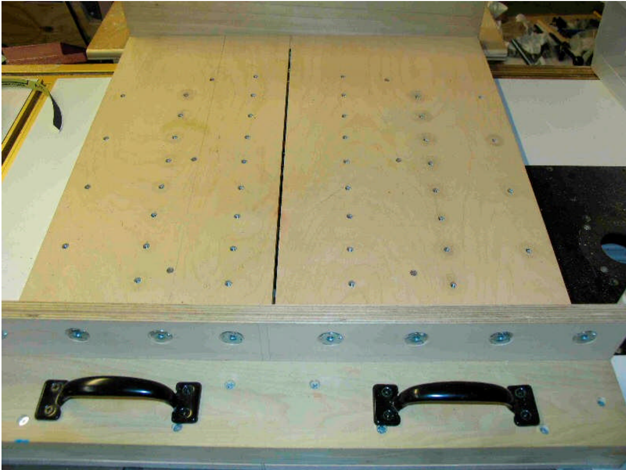
Figure 4 - Table Saw sled. Black handles keep my fingers out of harms way. Tee-nuts allow me to clamp whatever jigs, fixtures, or work hold-downs to the sled or to the back plate
