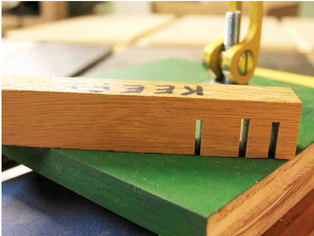
Figure 4 - On Left: Gauge Piece showing slices for my saw blades On Right: Gauge Piece with Inlay Slice
