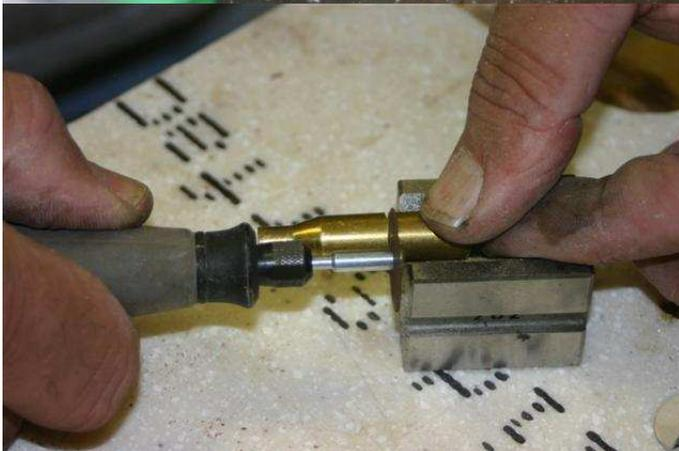
A Dremel tool with a cut-off disk can be used. Cut and turn until the brass is cut. Or, the brass can be sliced through, rotated and sliced again to finish the separation.
