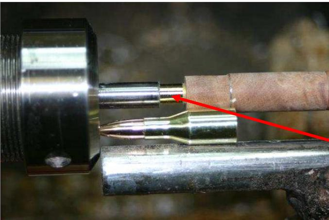
End of brass tube needs to be removed so it doesn't hit the end of the lead bullet.
