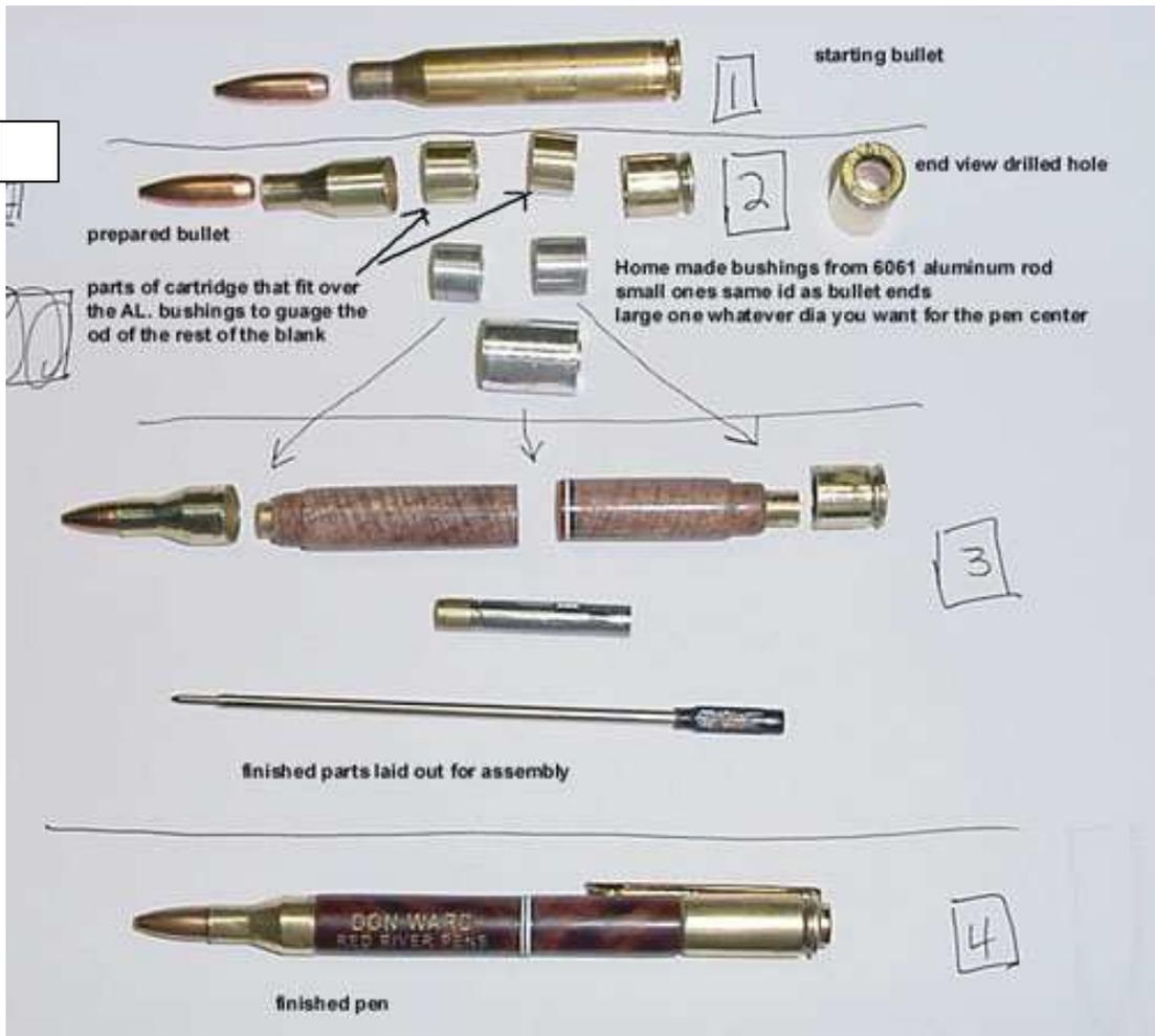
I have stopped using the homemade bushing. I turn the two parts on a 7mm pin chuck and I don't have the need remove the blanks repeatedly to measure.
