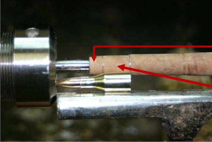
After rounding the blanks, mark critical areas to help guide next turning.
