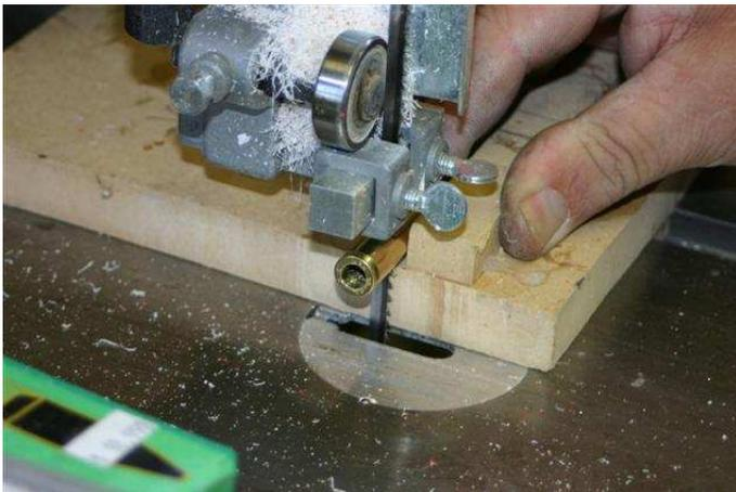
Cutting the brass on the band saw works. I use a blade that is too dull for wood. Hate to change blades so I don't use the band saw very often.
