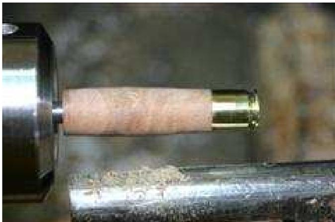
Finished tenon and fit. The two blanks are ready to mount on a mandrel and completed. Turn to desired shape, sand and finish.
