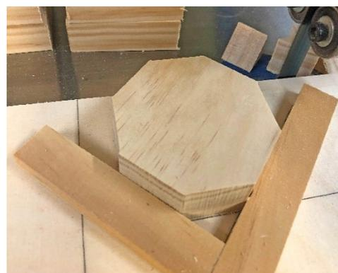
Find the center of one of the octagons by drawing lines to connect all of the opposing corners. The center will be where all of the lines cross each other.
