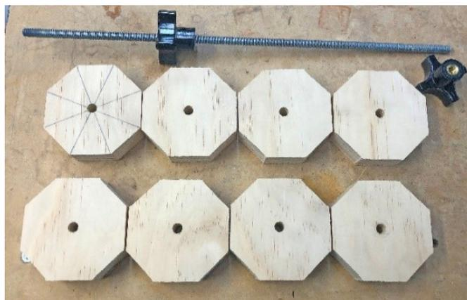
Apply glue to each set of 4 and re-align them on the threaded rod. Be sure to only apply glue to the inner surfaces of each set of 4 as you don't want to accidentally glue the two sets to each other. Also be sure to avoid using too much glue especially near the holes to prevent any squeeze out from blocking the holes. After gluing, use ¼-20 knobs (or nuts and washers) to clamp them together until the glue dries.
