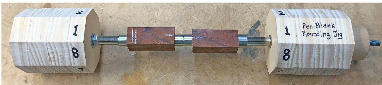
Lay the loaded jig on the bandsaw with one of the flat surfaces of the blank touching the outside surface of the bandsaw blade. Slide the fence on the bandsaw towards the blade until it just touches the jig and lock it into position.
