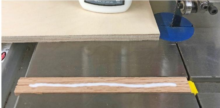
Position the plywood on top of the runner and apply some weight until the glue sets.
