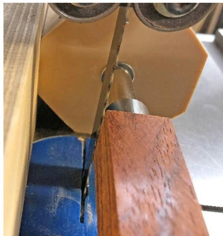
Move the jig back and turn the bandsaw on. After the saw is up to speed, carefully position the jig against the fence with the blade between the end of one of the blanks and the jig. Saw the blanks by moving the jig along the fence until both of the blanks have been cut.
