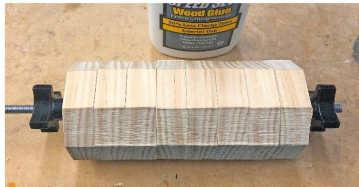
This is also an ideal time to label/number the sides of the jig. The two sections of the jig, each made out of a set of 4 octagons should both be labeled so that orientation between the two ends of the jig can be maintained when it is in use.
