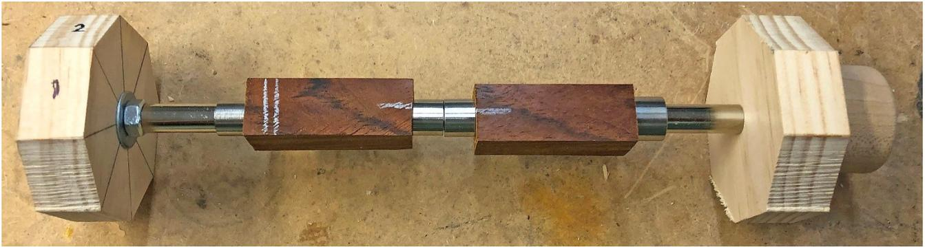
A very simple version of the jig can be built by using square blocks. Although the jig will be square and not octagonal, it will still work for cutting the corners off of blanks. When the blanks are loaded onto the jig, they must be strategically positioned so that the corners of the blanks are pointing up and towards the blade. This makes setting the distance from the blade be a little more difficult, but it should work as long as the blade does not hit any of the bushings.
