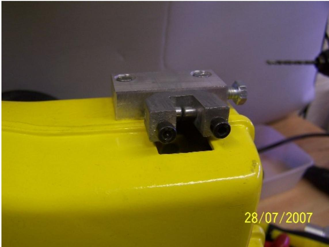
Finally was the mitre. Here I remove the existing slide and cut a piece of steel that just fits in the slot. I also made it longer than the table length to offer more support when using a jig like this one.
