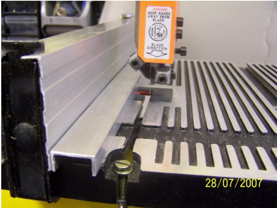
Next was the under table guides. The current position offered virtually no support for the blade. Here I made a little block to hold the guides and mounted it on the BSaw body. I could have taken it higher still, but then I couldn't tilt the table, but like this I can still tilt to 45 deg
