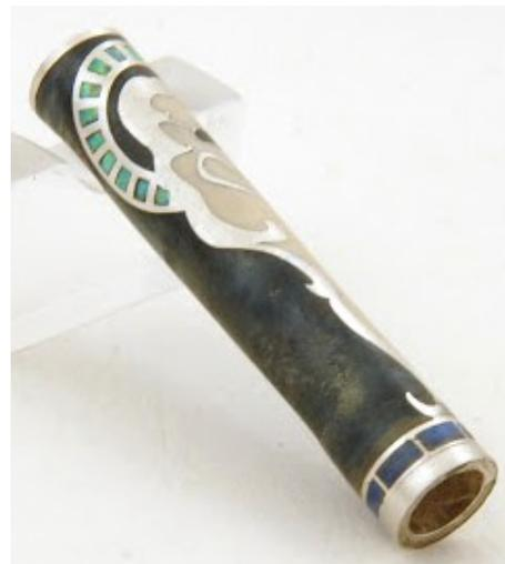
So, I had to take a ball burr and cut all the resin back off the pen. Sorry for the blurred picture of the blank after I removed all the resin.
