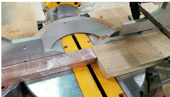
The slats against the stop are ready to be cut.
