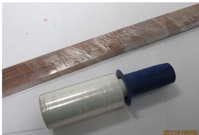
The slats are wrapped and ready for cutting into tiles.
