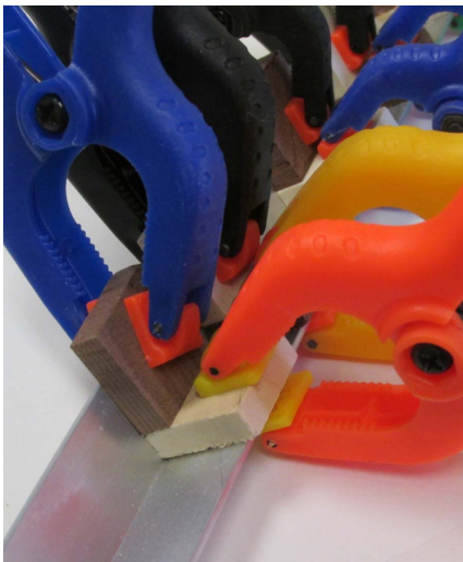
A close up of the slices clamped to the angle.
