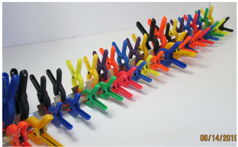
Pairs of slices glued and clamped to the angle using all of the clamps.
