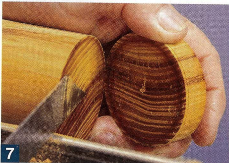
5 Make a tenon. Use the bevel side of a skew to make a series of light cuts, creating the tenon.
