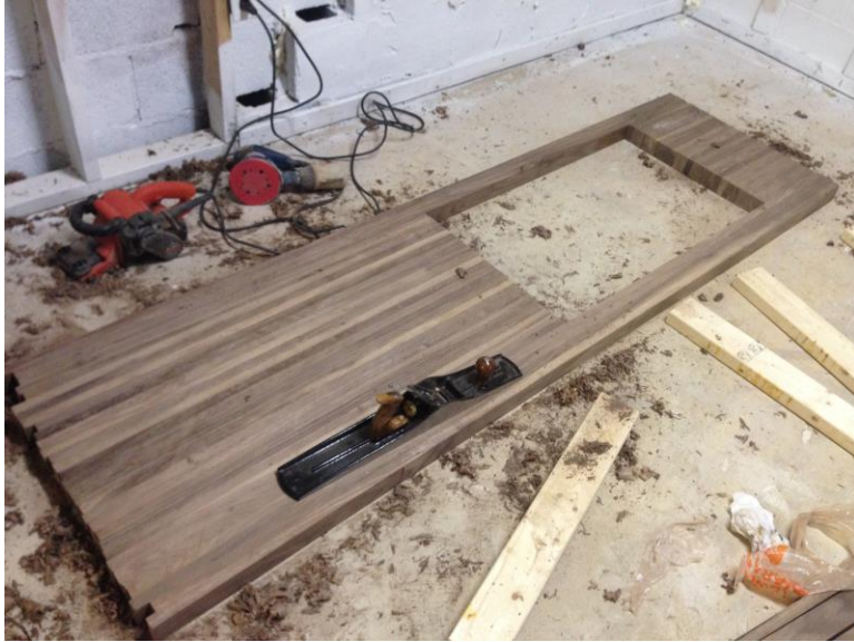
Knocking the glue off and flattening the stove side.
