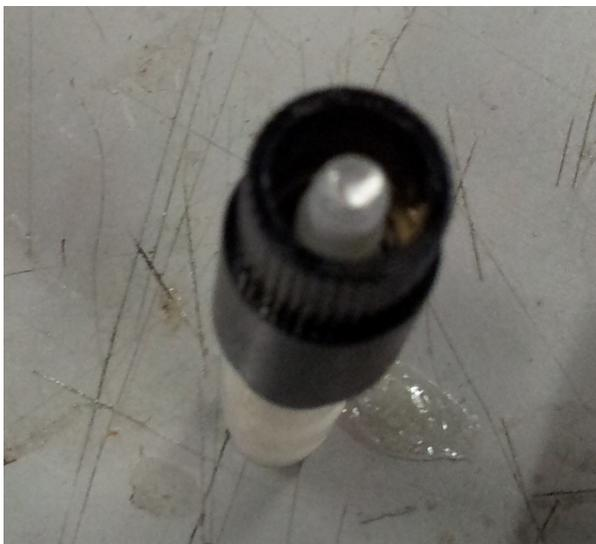
There will be a few moments when the air in the hole will not let the glue flow into it. Don't worry, just wiggle the paper clip slightly and the air bubble will break and you can spread the glue down into the hole. Just remember to not let the glue spill over onto the threads. Remove the paper clip quickly and set aside. Pick up the nail and drop it into the hole.
