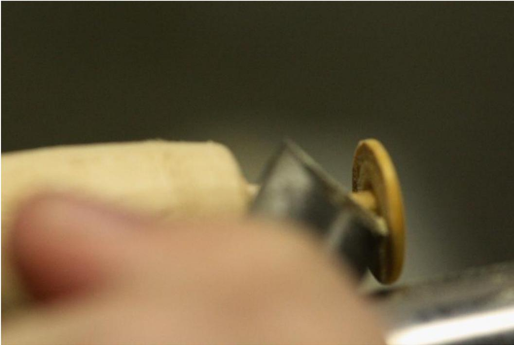
Here's the finial after the tenon was checked to be the proper diameter.
