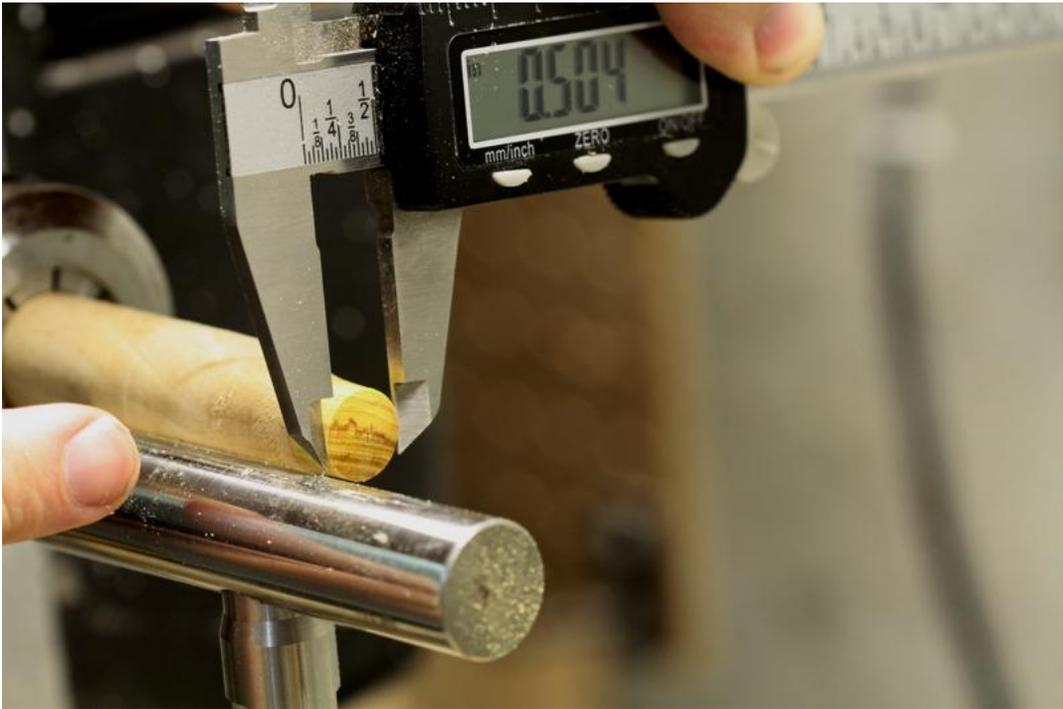
With a thin parting tool, begin to part a groove, leaving only the last 1 millimeter or so at full diameter. Do not part down all the way yet.
