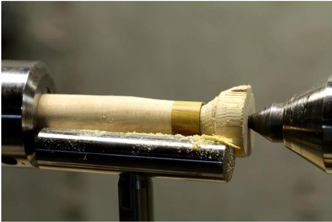
Remove the tailstock and face the end with an arcing cut with the skew. This is a difficult cut and should be practiced on scrap first. When mastered, you can produce conical shavings and a glass smooth surface. If the skew skates across your work, don't worry... you should have enough meat left to clean them up. You may need to make a few cuts until you are happy with the shape of the profile.
