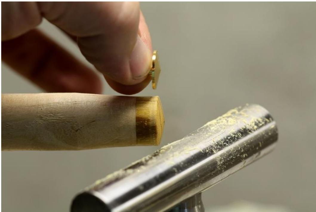
Take the diameter down further, cleaning up any tearout or skate marks from the previous step. Keep checking with calipers until the end matches the diameter of the stock finial.
