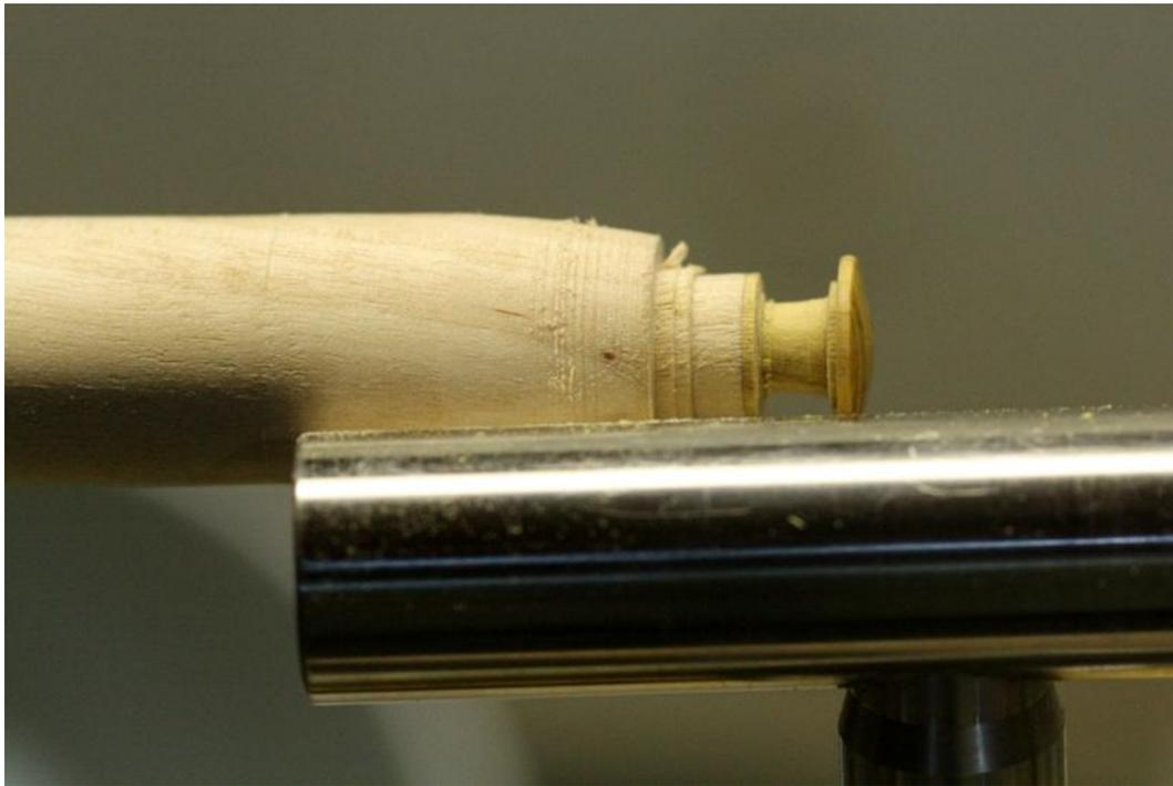
Once I create some clearance room, I like to take the final cuts with the toe of a small skew.
