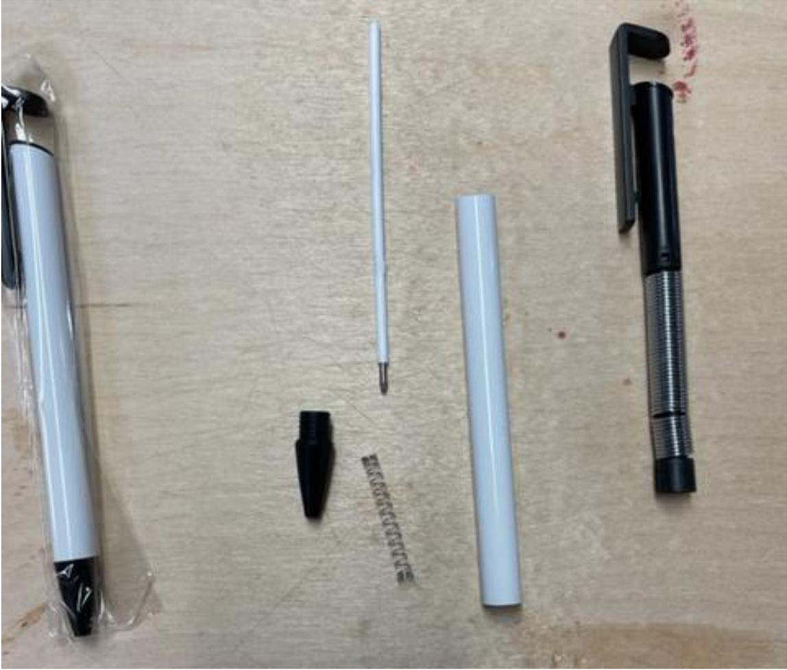
You will find a 3/8 brass tube fits very nicely inserted into it. The sublimated tube is aluminum and the wall thickness is only .012.
