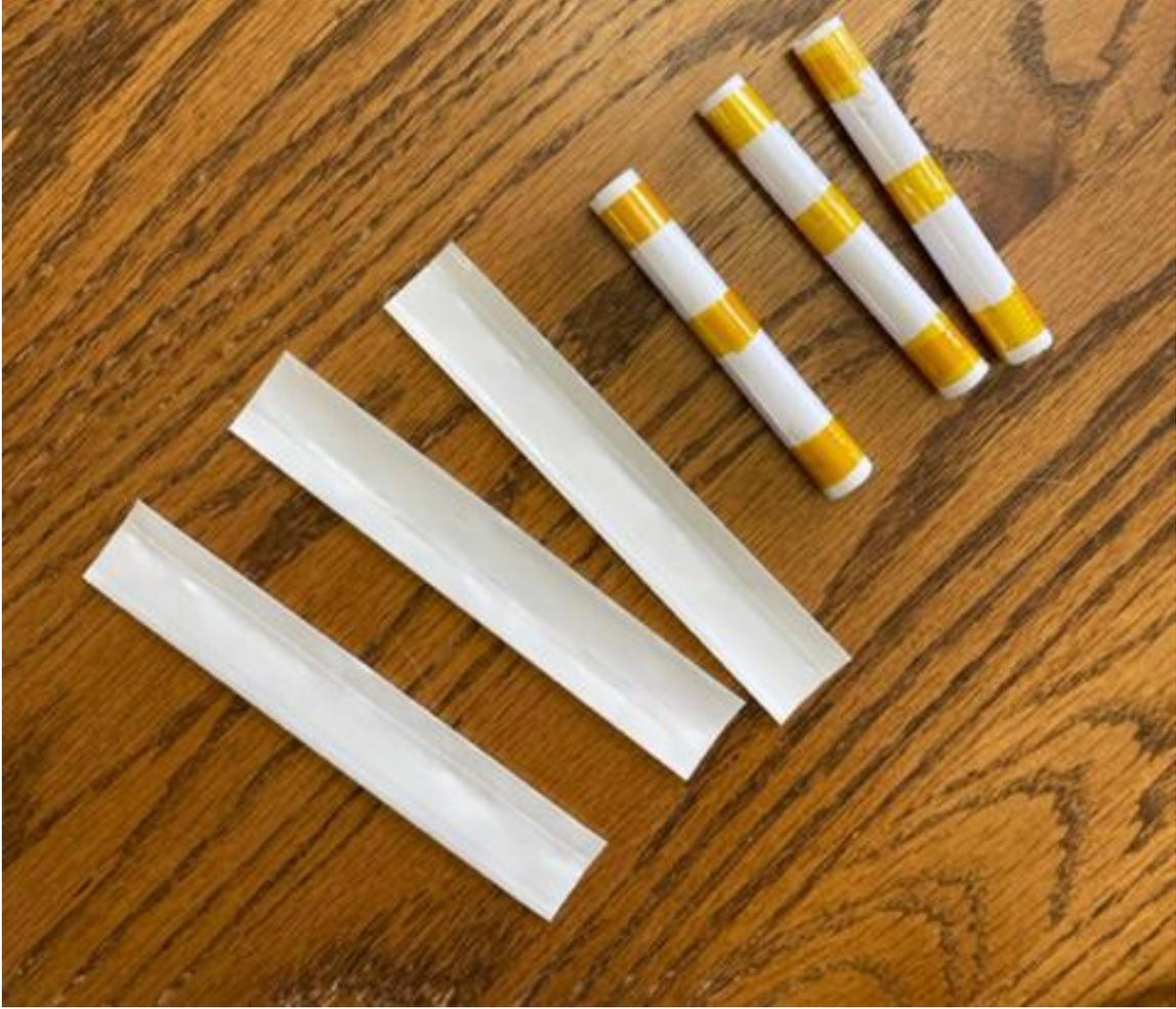
Step 7: Insert the wrapped tubes into the heat shrink tubes.
