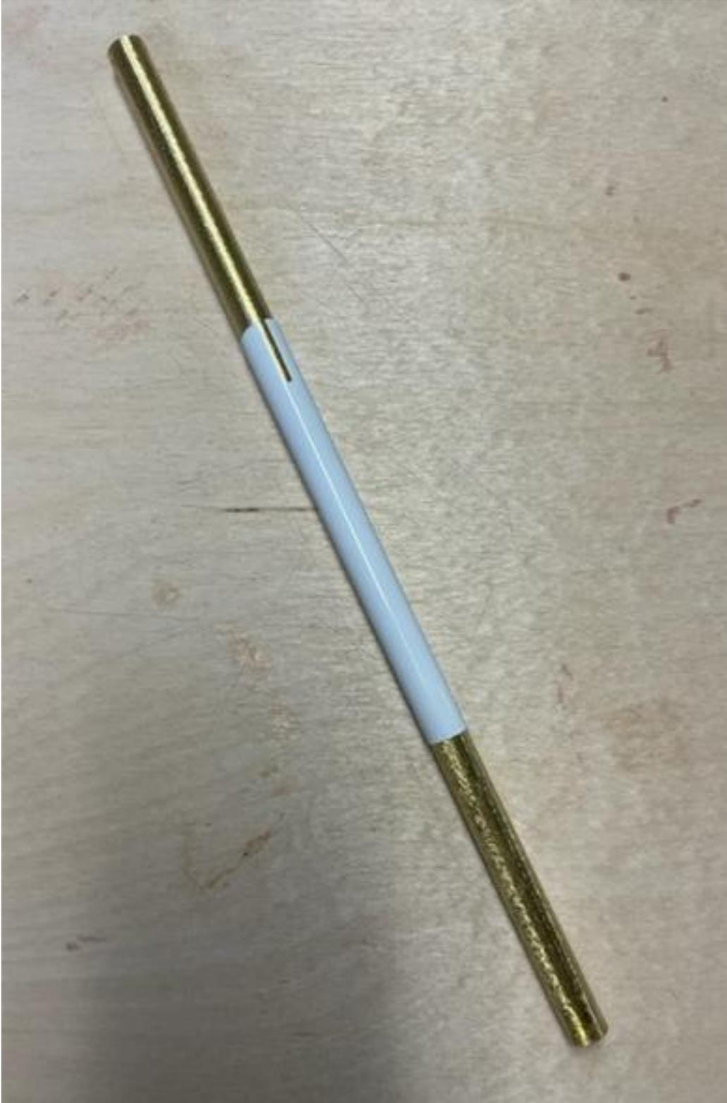
Step 5 : Cover the white sublimation tube with painters tape and cut it just slightly longer than the brass tube you are going to glue inside it.
