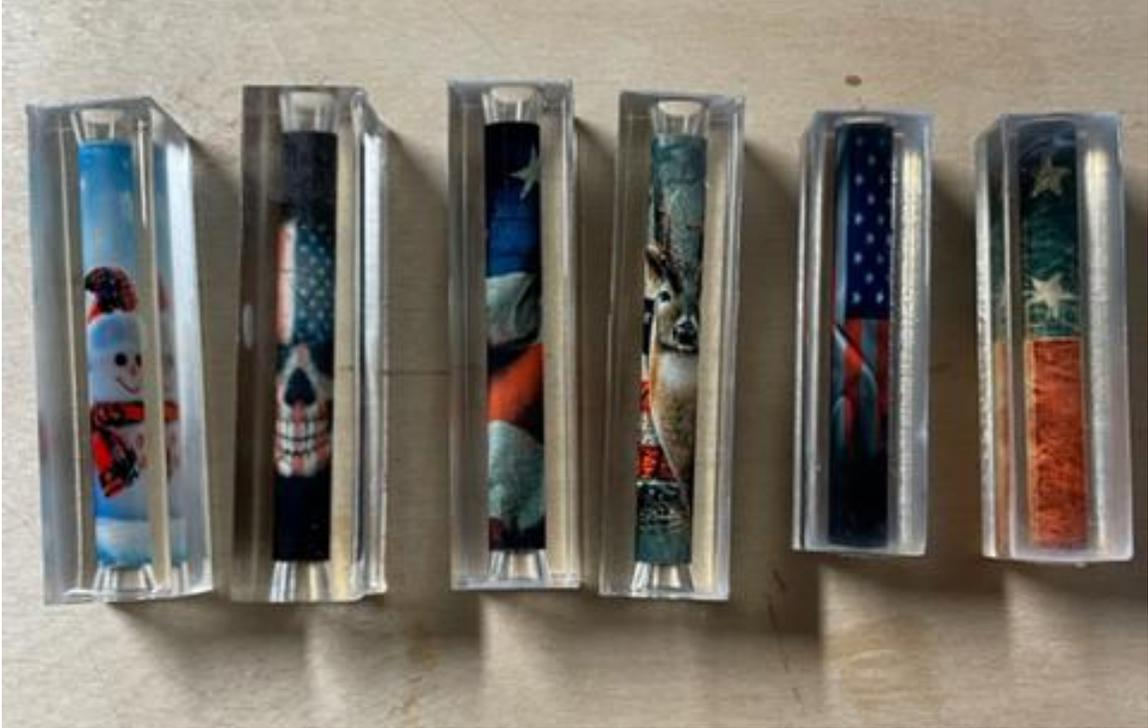
If you want to go the route of applying the sublimation material on the brass tubes, you will need to first paint them with high temperature white paint and then follow the directions on the sublimation coating bottle. Also make sure you buy the kind for hard substrates.
