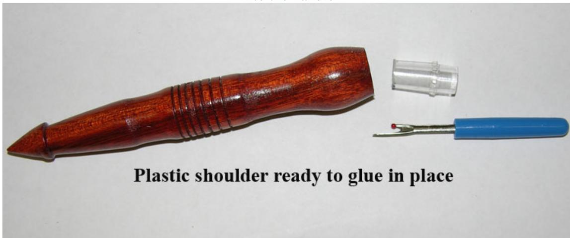
Once the clear plastic is glued into the handle, (tapered end into it) allow it to sit, this of course depends on the type adhesive you choose, I would recommend NOT using Gorilla glue, Epoxy or thick CA will do just fine.
