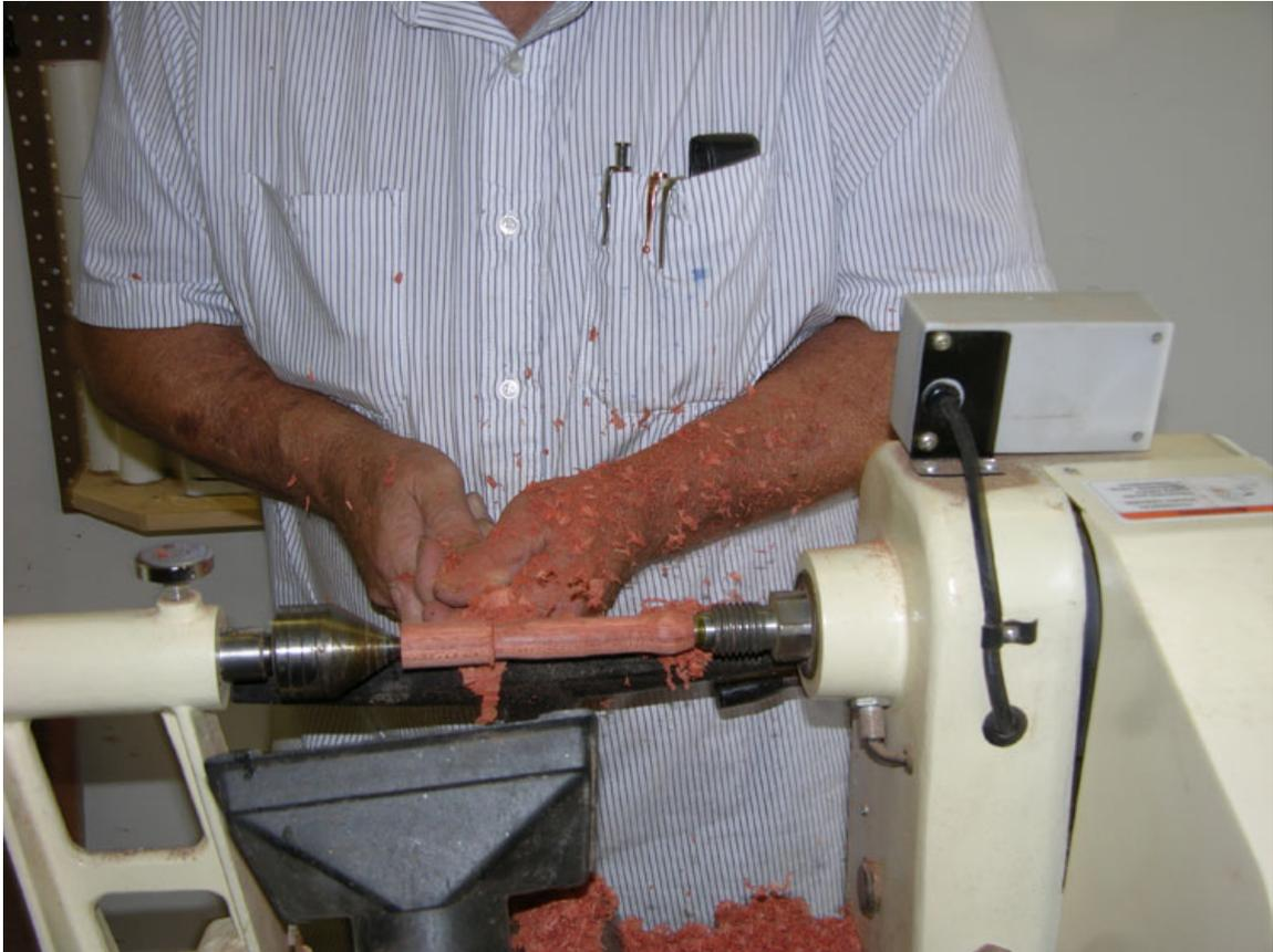
Now you can either turn your blank between centers, just don't chuck up so tight that you break the blank, or you can use a spur center instead of a 60 degree dead center, since most lathes come with a spur you probably will want to use that, but for this I used a 60 degree dead center.
