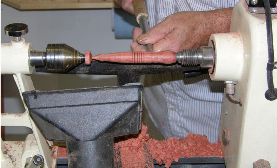
I also like to cut pinnacles and artsy finials on the tool handle as well as some coves with a Round 1 tool or a small spindle gouge and rings with a skew which make for easier grip.
