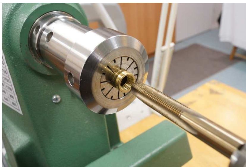
Threaded to 3/8" 24 NF Threads
