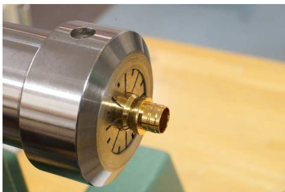
Bolt Chamber Installed in Collet
